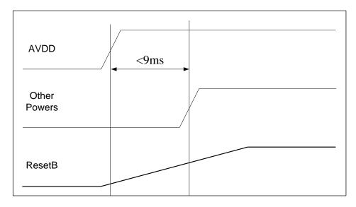
Figure 2: Power-on Reset Function's Sequence on board
