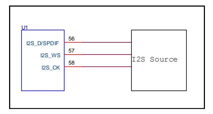
Figure 10: CH7053A I2S Input Pins
