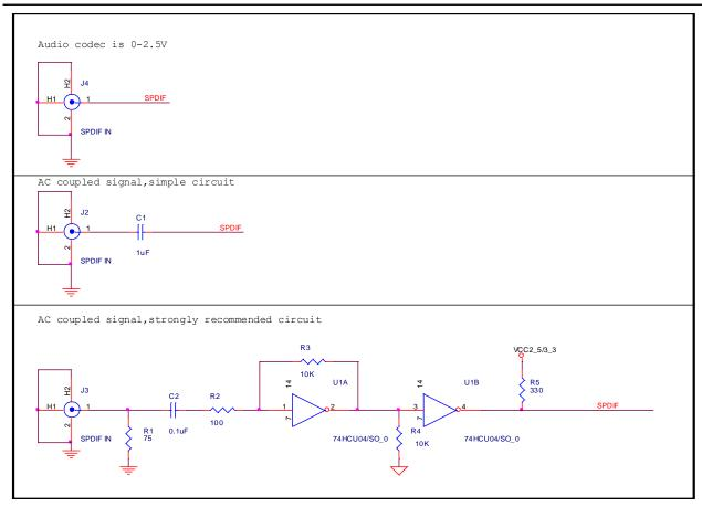
Figure 9: SPDIF pin of CH7053A
