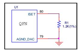
Figure 4: ISET pin connection
