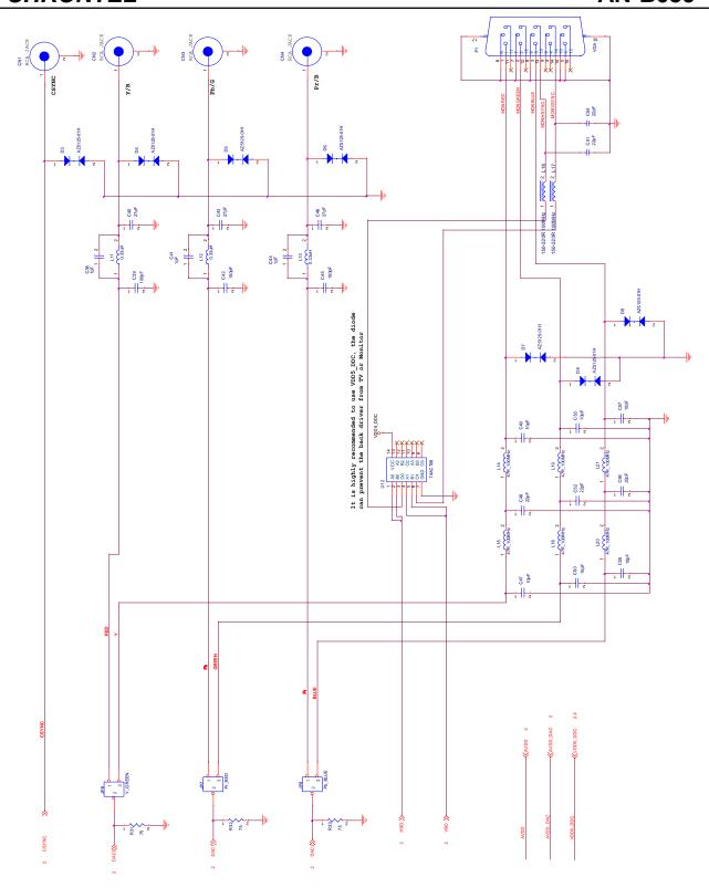
(b) YpbPr, RGB+Csync and VGA output
