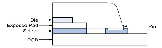
Figure 14: Cross-section of exposed pad package
