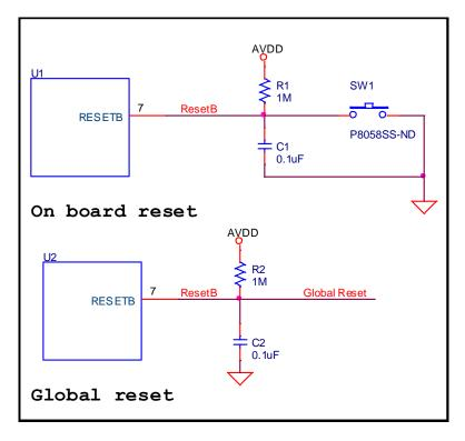
Figure 5: RESETB pin connection
