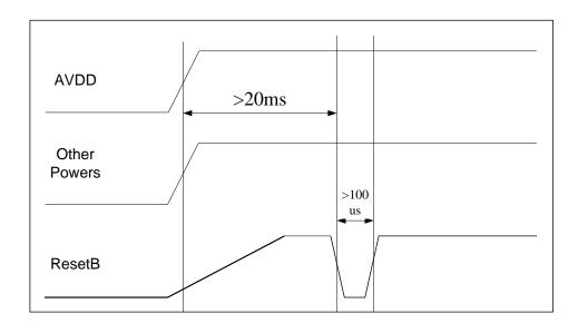
Figure 3: Power-on Reset Function's Sequence external global reset
