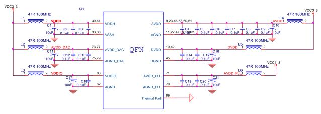
Figure 1: Power Supply Decoupling and Distribution
