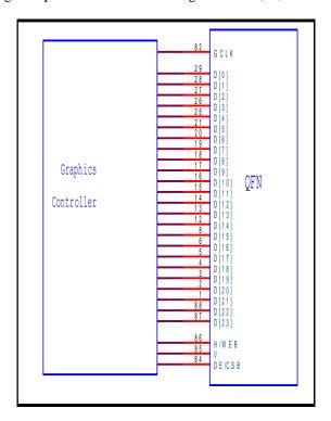
Figure 8: CH7053A Data Input Pins
