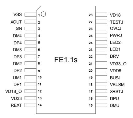
Fig. 2: SSOP-28 Pin Assignment
