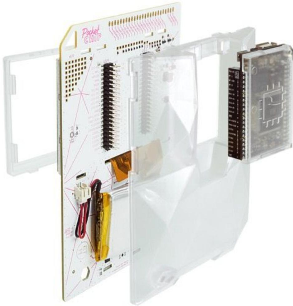
PocketC.H.I.P. is designed to be easily taken apart since there are no screws used in the assembly.
