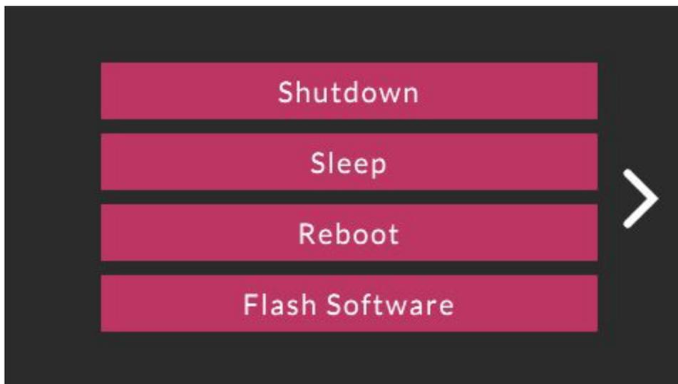
Sleep is a low-power state that saves battery, and also saves you time, since it's faster for PocketC.H.I.P. to wake from sleep than to boot from a powered-off state.
