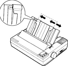
4. Slide a sheet of paper down firmly between the edge guides until it meets resistance.
