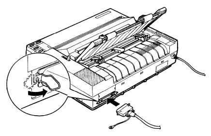
**Note:** If your cable has a ground wire, connect it to the ground connector beneath the interface connector.
