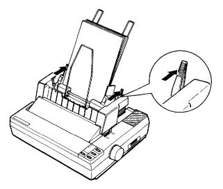
A new sheet of paper loads automatically whenever a printable character or line feed command is sent to the printer while the ON LINE light is on.
