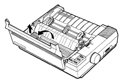
2. Slide the print head to the middle of the printer. Then open the paper tension unit cover.
