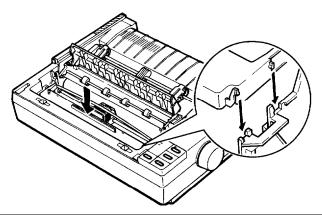
**Note:** Press lightly on both ends of the cartridge to make sure the plastic hooks are properly seated.
