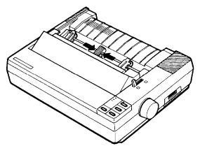
5. Open both sprocket covers. Fit the first three holes in the paper over the pins of both sprockets.
