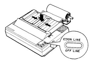
**Note:** To tear off paper after printing, set the printer off line, press the LINE FEED button to advance the paper, then tear off the paper against the tear-off edge of the printer cover.
