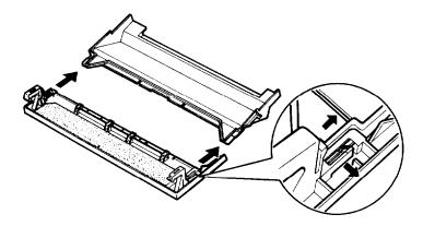
10. Attach the tractor cover to the front half of the printer cover.
