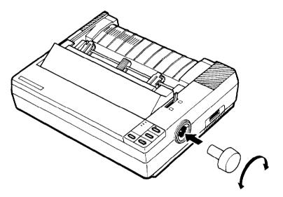
2. Push firmly on the platen knob until it fits against the printer case.
