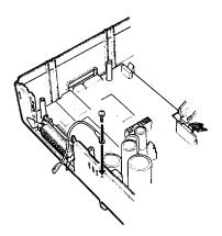
2. Carefully insert the pins on the optional interface board into the mating connector on the main board; then secure the board with the three screws provided.
