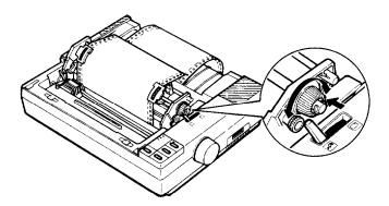
*8.* Make sure that the paper-release lever is set forward to the continuous paper position.
