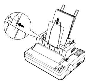
3. Press the LOAD/EJECT button to load the sheet.
