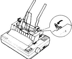
2. Slide the left paper guide to where the fin **on** the edge guide aligns with the arrow on the front panel. Next, slide the right paper guide to roughly match the width of your paper.
