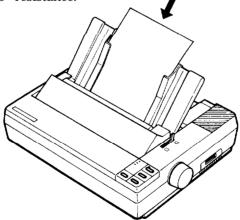
**CAUTION:** Run the self test using paper wider than A4 (210 mm or 8½ inches) or letter size (216 mm or 8½ inches), to prevent the print head from printing directly on the platen.
