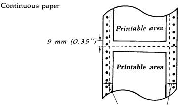
13 mm (0.51 inch) or more (both sides) when the 101 mm to 242 mm (4 to 9.5 inch) width paper is used. 26 mm (1.02 inch) or more (left side) and 24 mm (0.94 inch) or more (right side) when the 254 mm (10 inch) width paper is used. Envelope
