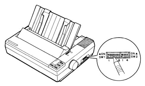
The new DIP switch settings take effect when the printer is turned **on**.
