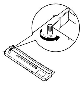
4. Hold the ribbon cartridge by its handle and push it firmly down into position, making sure the plastic hooks fit into the slots.
