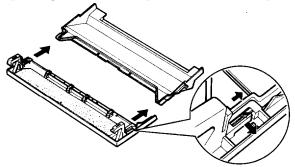
3. Attach the cut-sheet feeder cover to the front half of the printer cover.
