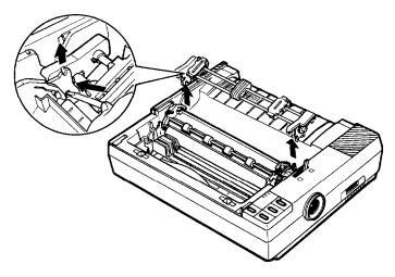
5. To remove the upper case, first position the printer so that its front extends slightly over the edge of a table, allowing access to the openings on the front of the underside of the printer.
