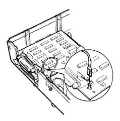
4. If you have the #8148 or #8165 interface boards, set the interface DIP switches according to the accompanying manual.
