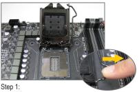
Gently press the CPU socket lever handle down and away from the socket with your finger. Then completely lift the CPU socket lever and the metal load plate/plastic cover will be lifted as well.
