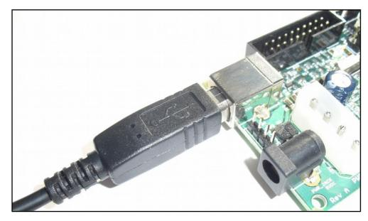
8. Attach the USB cable to KryoFlux and then attach it to your computer. Do not use a USB hub!
