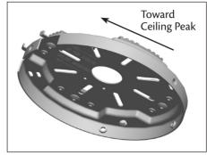
For Angled Ceilings: Be sure to orient the ceiling plate so that the two tabs are pointing toward the ceiling peak.
