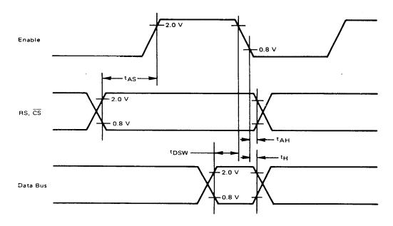
FIGURE 6 - BUS TIMING TEST LOAD
