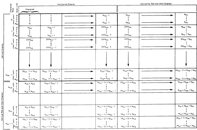
NOTE 1 The initial MA is determined by the contents of start address register, R12/R13. Timing is shown for R12/R13 = 0. Only Non-Interlace and Interlace Sync Modes are shown.
