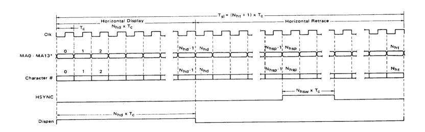
\*Timing is shown for first displayed scan row only. See Chart in Figure 16 for other rows. The initial MA is determined by the contents of Start Address Register, R12/R13. Timing is shown for R12/R13 = 0.
