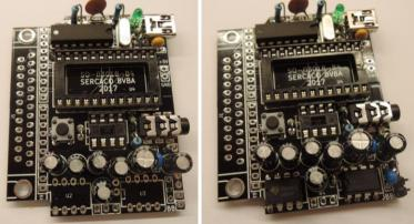
At this stage you can already test if the 5V power works fine : if there are no shorts , the green led should burn when you plug the board on an usb cable to your 5V power source. If this works, add the remaining components.
