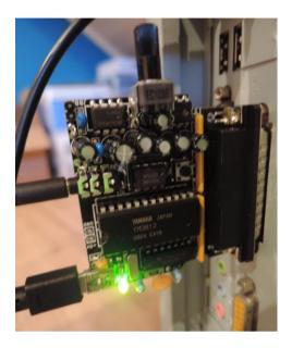
Now using the test program 'opl2test', you should hear some music. Adjust the potentiometer until you hear a suitable volume.
