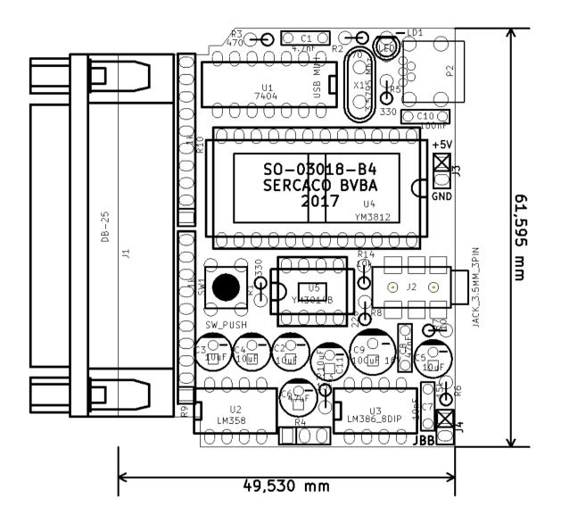
For LD1, C2,C3,C4,C5, C6, C9, C11 : take care to respect the polarity. The negative side is marked with - on the PCB.
