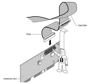
8 Install the accelerator card into the 16-bit expansion slot by pushing <u>firmly</u> on the accelerator edge until it "clicks" into the slot; secure with a screw.
