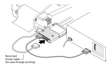
7 Connect the external power supply to your power source and the tape drive. When the drive is first plugged in, the tape drive activity light flashes and then turns OFF. The power light remains on.
