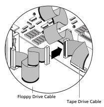
15 Feed the free end of the tape cable out through the open bay of the computer.
