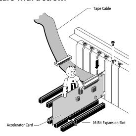
9 Thread the tape cable through the bay opening where the tape drive will be installed.
