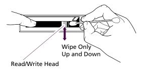
Caution: No other maintenance procedures are authorized by Iomega. Attempting to service the drive in any other way will void the warranty. (NEVER touch the read/write head or any other internal part of the drive with your fingers.) QIC-80 cleaning cartridges are NOT compatible with QIC-3020 Travan drives and will damage the read/write head.
