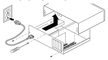
3 Locate a vacant 5<sup>1</sup>/<sub>4</sub>-inch horizontal drive bay. Remove the plastic cover and, if necessary, the metal shield.
