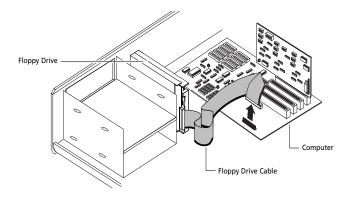
13 Now plug the tape cable onto the same connection from which you just removed the floppy drive cable. Be sure to maintain the stripe orientation.
