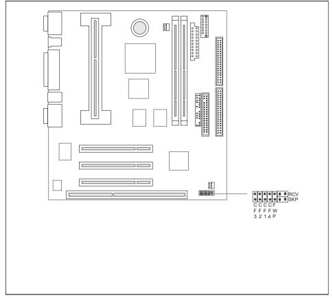
Jumper SKP = May not be inserted Jumper RCV = System BIOS recovery Jumper FWP = Write protection for floppy disks Jumpers CF3, CF2, CF1, CF4 = Clock speed
