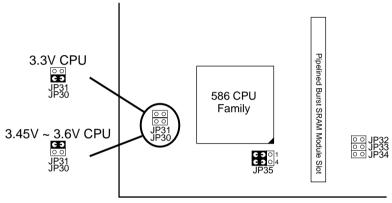
Figure 2–2–1. Single Voltage CPU
