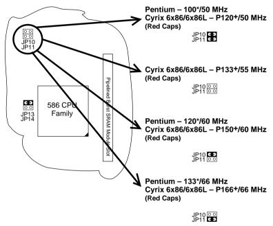
Figure 2–1–2. CPU Jumper Settings
