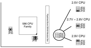
Figure 2–2–2. Dual Voltage CPU
