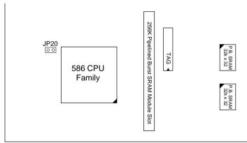
Figure 2–3–1. 256K Pipelined Burst Cache Configuration
