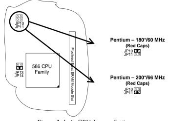
*Figure 2–1–4. CPU Jumper Settings*
