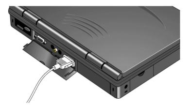
The OmniBook automatically recognizes and activates the external monitor. The built-in display normally turns off to conserve power and backlight life—but if you keep it on, you may notice a slight dimming while the external display is connected.
