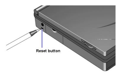
If the reset button has no effect, remove the battery and ac adapter and press the reset button—then install the battery or plug in the ac adapter and try pressing the reset button again.
