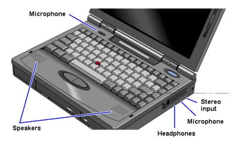
You can also plug in an external microphone, external speakers or headphones, and a stereo input source—such as a CD player.
