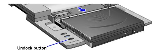
The OmniBook closes down any connections to the docking system and ejects the computer.
