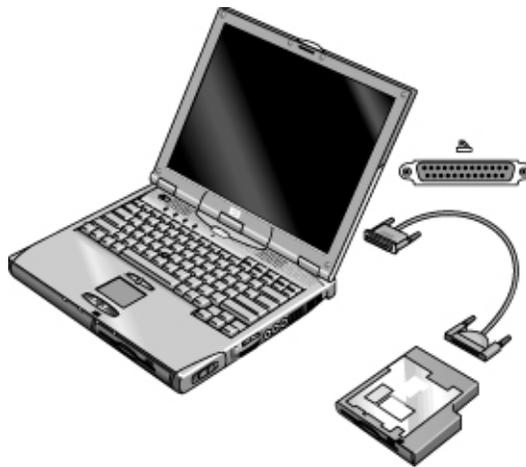
Before disconnecting the floppy disk drive, use the icon in the taskbar to stop the drive, or else shut down the computer. See “To replace a plug-in module” on page 55.
