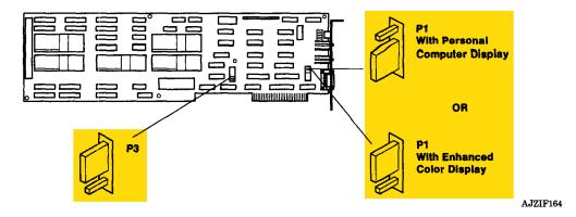
Use the charts on the following pages to correctly set the switches for the display attached to the Enhanced Graphics Adapter.
