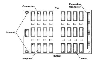
2. Install each module with the notch facing the bottom edge of the card, as shown in the following drawing:
