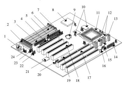
Keyboard connector: The default is AT-compatible keyboard. The P/2-compatible mini-DIN keyboard connector is optional.
