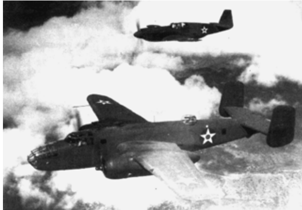
B-25D in formation with an A-36. The A-36 Apache was the early variant of the P-51 Mustang. Equipped with an Allison engine, the A-36 was used as a dive bomber/attack craft in Italy. Later, a British Marlin engine was mated to the airframe, creating the P-51B Mustang. (Courtesy Foto Consortium)
