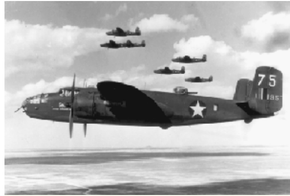
The versatile B-25. This version, a B-25D, has a glass nose. B-25s were often field-modified to carry up to eight machine guns in the nose. (Courtesy Bob Lawson)
