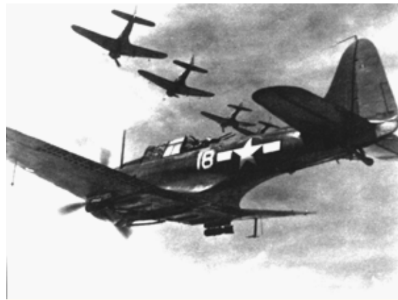
An SBD carrying two small 100-pound bombs. (Courtesy National Air & Space Museum, Smithsonian Institution)
