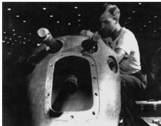
A worker assembles part of a P-38 nose section. Note the four .50 calibre guns along the top and the 20mm cannon in the center. (Courtesy National Air & Space Museum, Smithsonian Institution)
