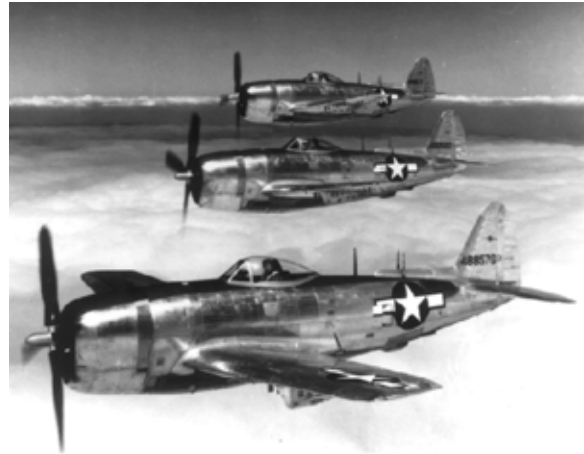
Late war P-47Ds with the bubble canopies. These canopies dramatically improved the pilot's rearward vision. (Courtesy Bob Lawson)
