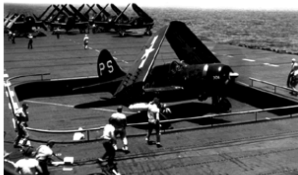
A late war photo of an SB2C. Note the hardpoints on the wings for rockets. (Courtesy Bob Lawson)
