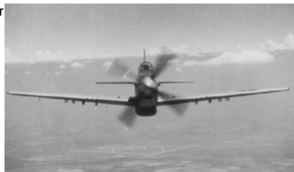
A Mustang with rocket hardpoints on the wings. It was a mediocre fighter-bomber since its liquid-cooled engine was highly vulnerable to enemy ground fire. (Courtesy Foto Consortium)
