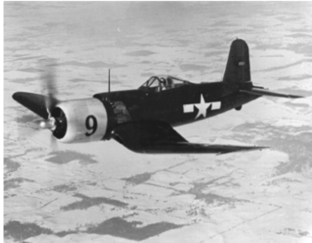
The XF2G in flight. Designed specifically as an anti-kamikaze fighter, the F2G initially carried only four 50 caliber machine guns. (Courtesy Bob Lawson)
