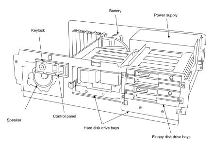
Figure 9 The IBM AT unit interior.
