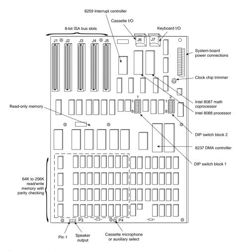
Figure 3 The IBM PC motherboard.
