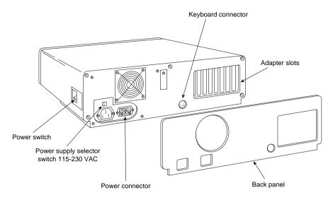
Figure 10 The IBM AT rear panel.
