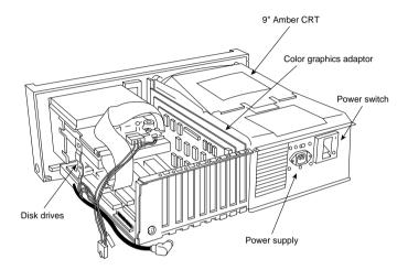
Figure 8 The IBM Portable PC interior.
