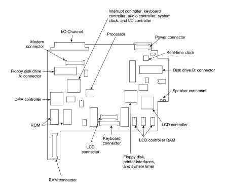
Figure 4 The PC Convertible motherboard.
