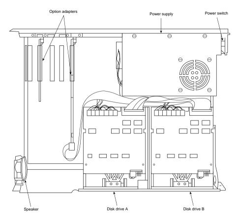
Figure 1 The IBM PC interior view.
