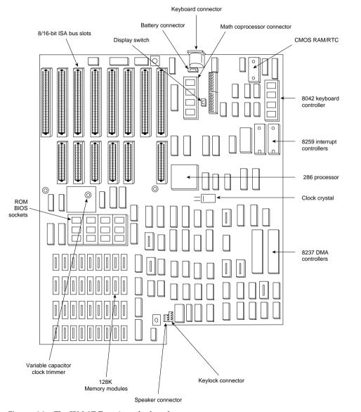
Figure 11 The IBM AT Type 1 motherboard.
