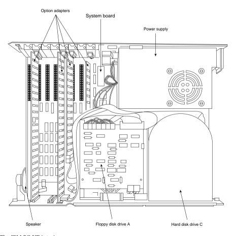
Figure 5 The IBM PC XT interior.
