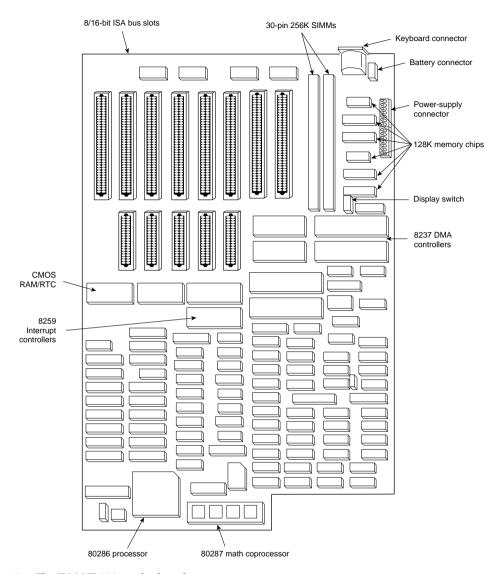
Figure 14 The IBM XT-286 motherboard.
