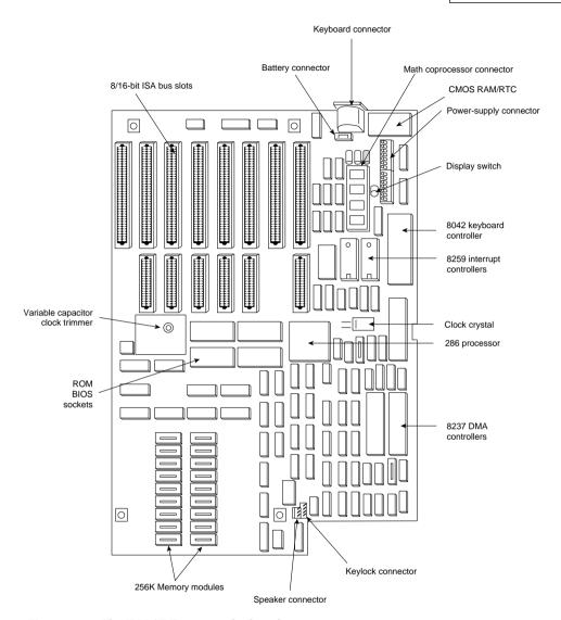
Figure 12 The IBM AT Type 2 motherboard.
