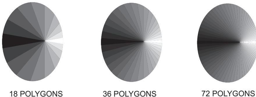
**Figure 6-8** *Flat Shading*
