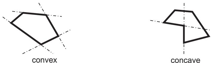
**Figure 2-10** *Concave and Convex Polygons*
