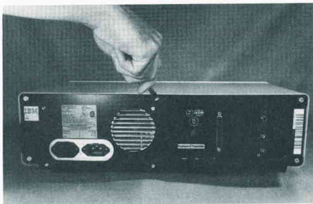
Fig. A-2. Remove these screws to disassemble the IBM PC.
