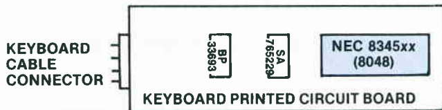
Fig. 4-38A. Chip location guide. This is a guide to help you find the 8048 IC inside the keyboard.
