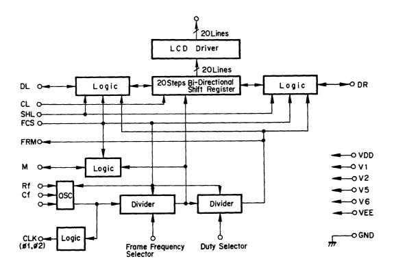
Figure 4-22. HD44103 Internal Logic Diagram
