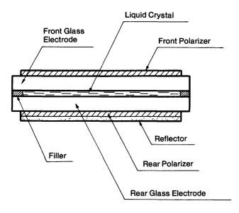
Figure C-16. Construction of LCD Panel
