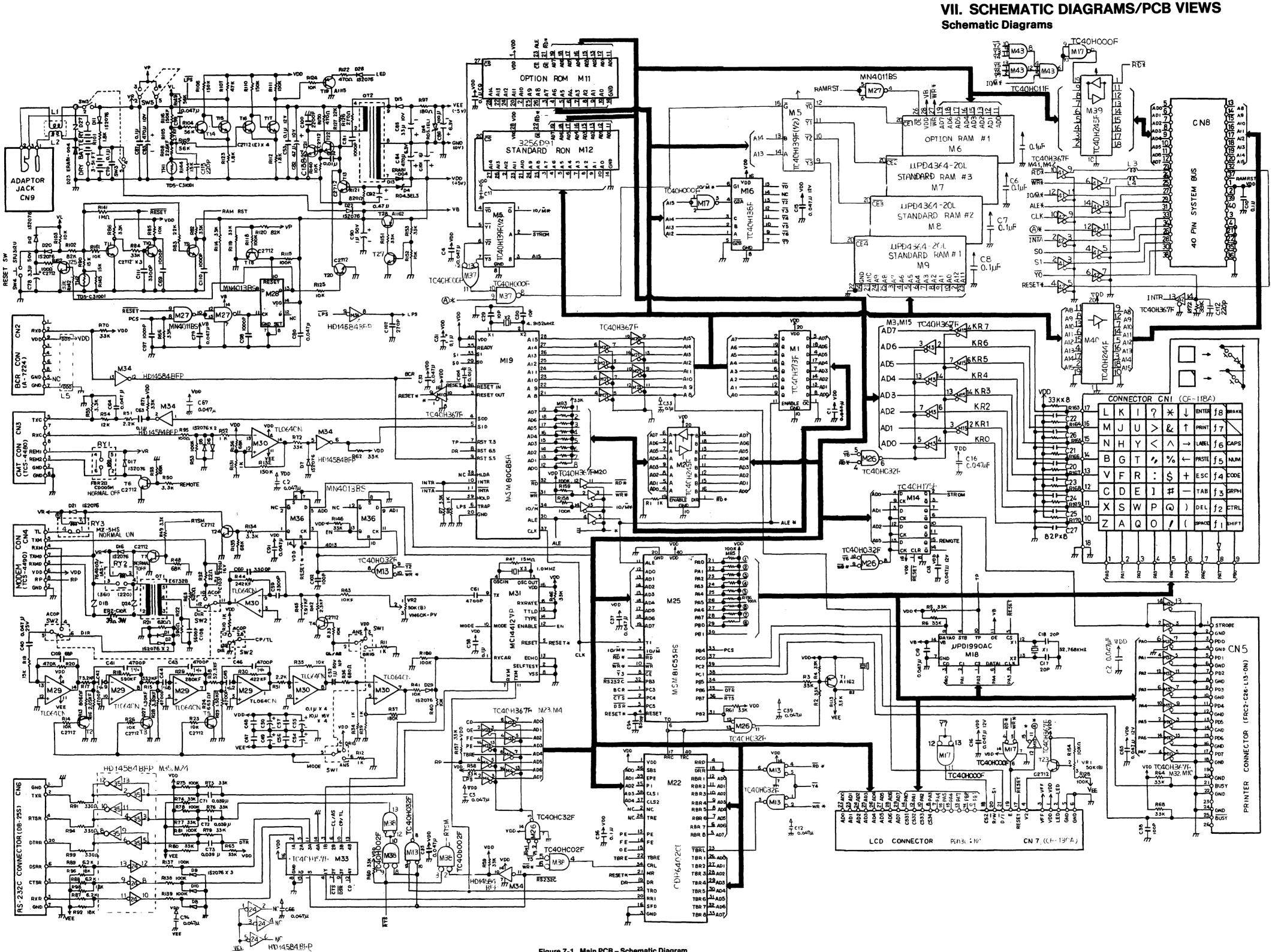
Figure 7-1. Main PCB – Schematic Diagram
