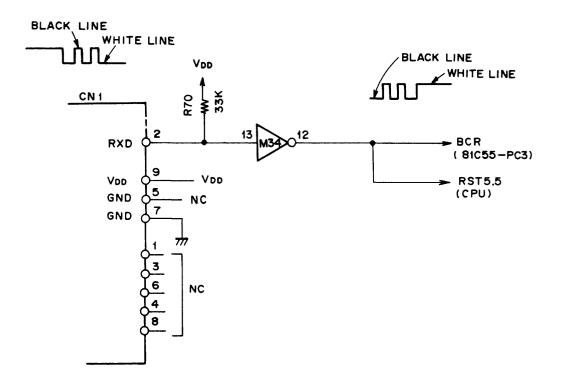
Figure 4-10. Bar Code Reader Interface Circuit
