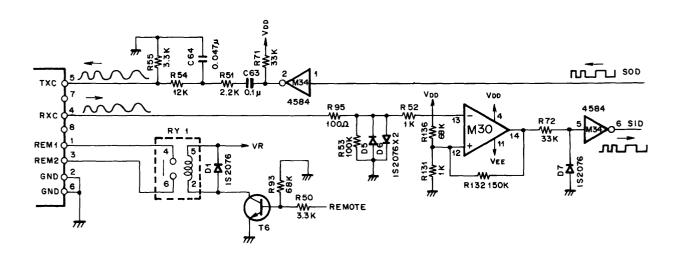
Figure 4-8. Cassette Interface Circuit
