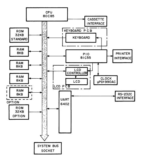
Figure 4-2. System Block Diagram
