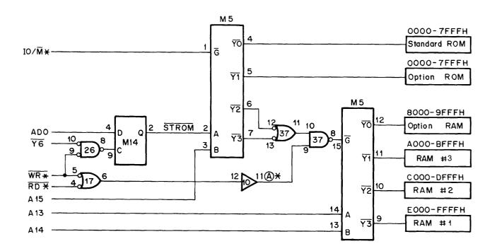
Figure 4-5. Address Decoding and Bank Selection Circuit
