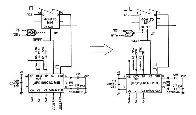
Figure 4-12. Time Set Sequence of  $\mu$ PD1990AC
