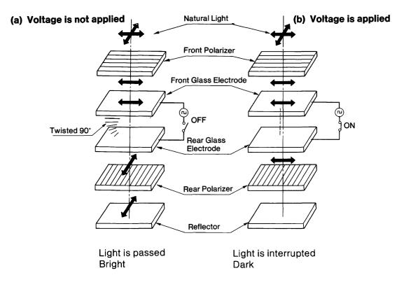
Figure C-17. Operation Theory of LCD Panel
