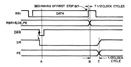
Figure C-13. Receiver Timing
