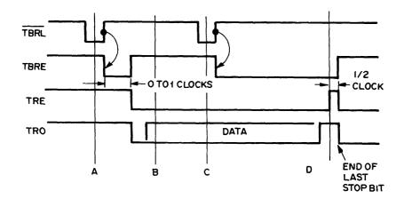
Figure C-14. Transmitter Operation
