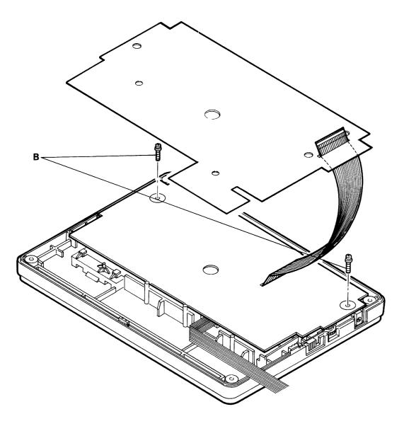
Figure 2-3. Main PCB Removal
