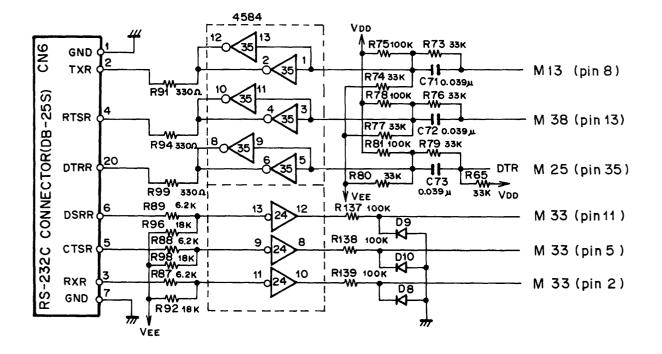
Figure 4-16. RS-232C Interface Circuit
