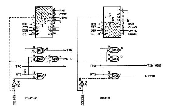
Figure 4-15. RS-232C/MODEM Selection Circuit
