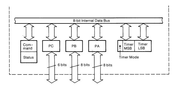
Figure C-7. Internal Register of 81C55
