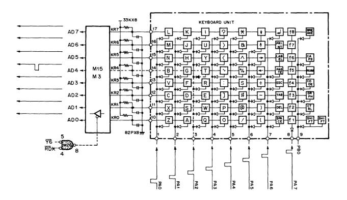
Figure 4-7. Condition of Pressing "T" Key
