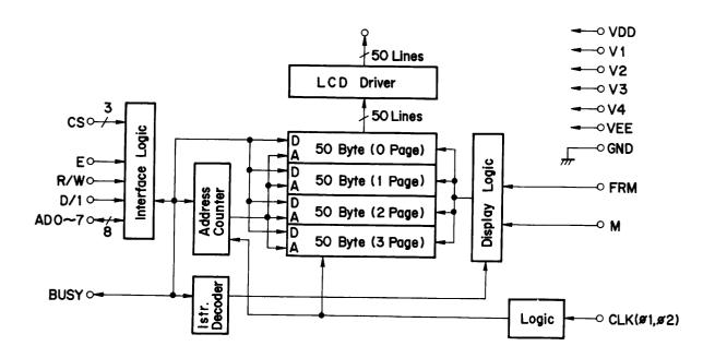
Figure 4-23. HD44102 Internal Logic Diagram
