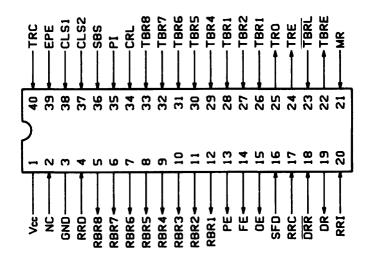
Figure C-12. Pin Configuration of 6402
