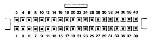
Figure B-2. System Bus Connector
