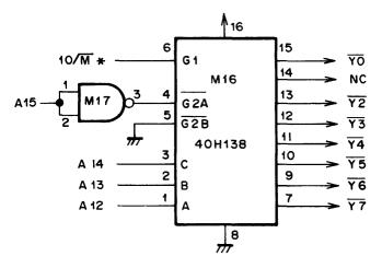
Figure 4-6. I/O Address Decoding Circuit
