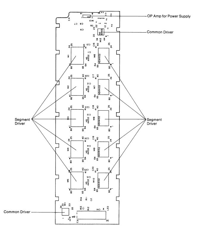
Figure 1-5. LCD PCB
