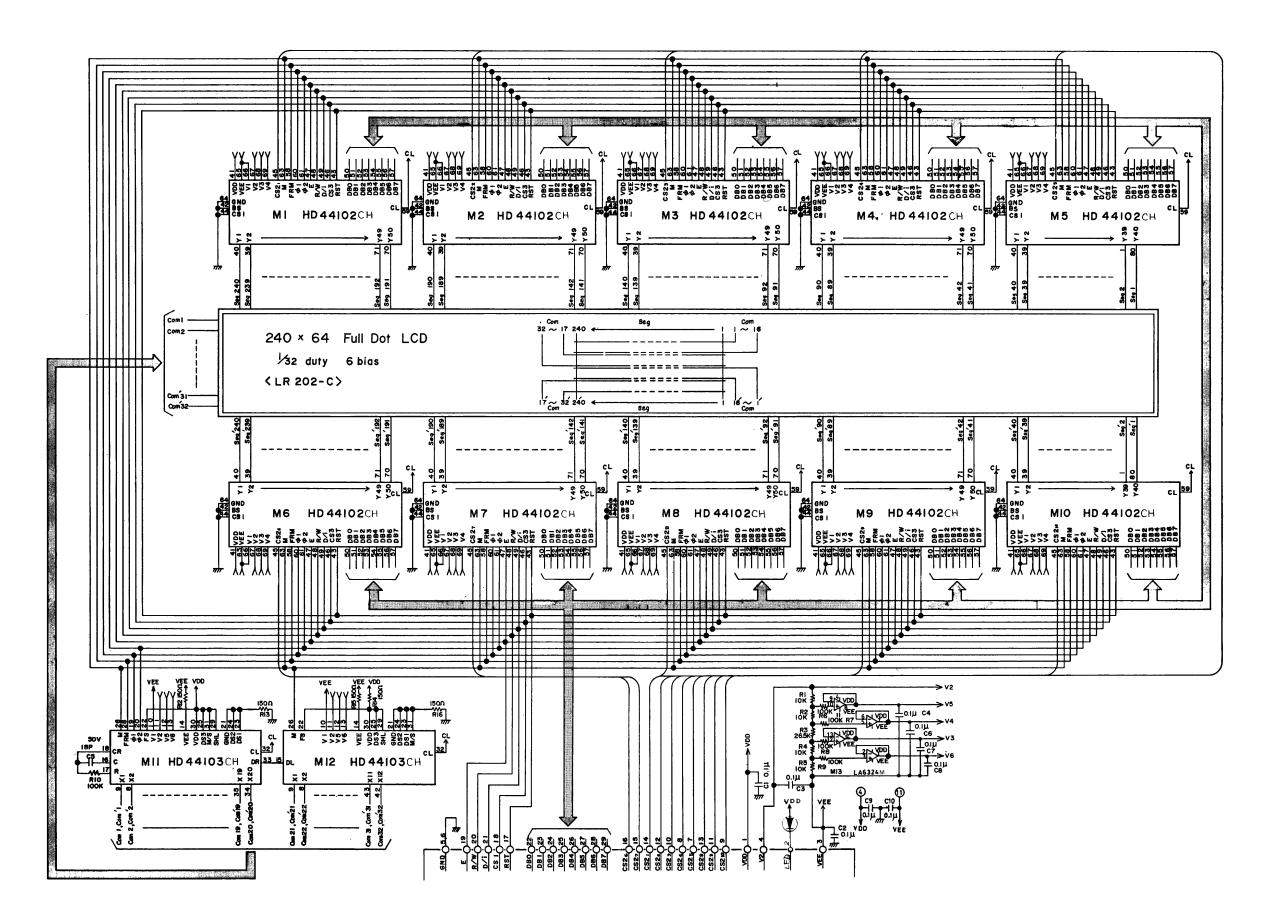
Figure 7-2. LCD PCB – Schematic Diagram
