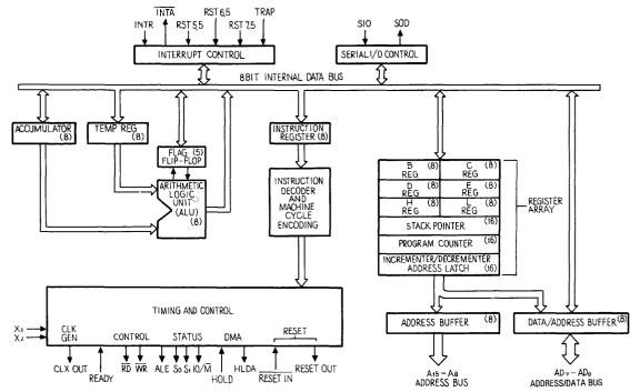
Figure C-1. Functional Block Diagram
