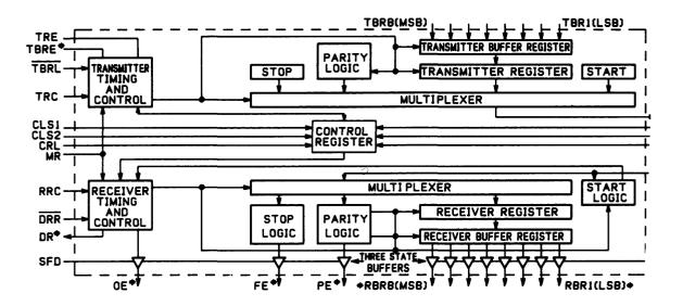
Figure C-11. Functional Block Diagram
