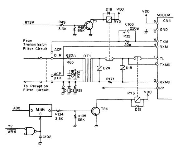
Figure 4-21. MODEM Connector Interface Circuit
