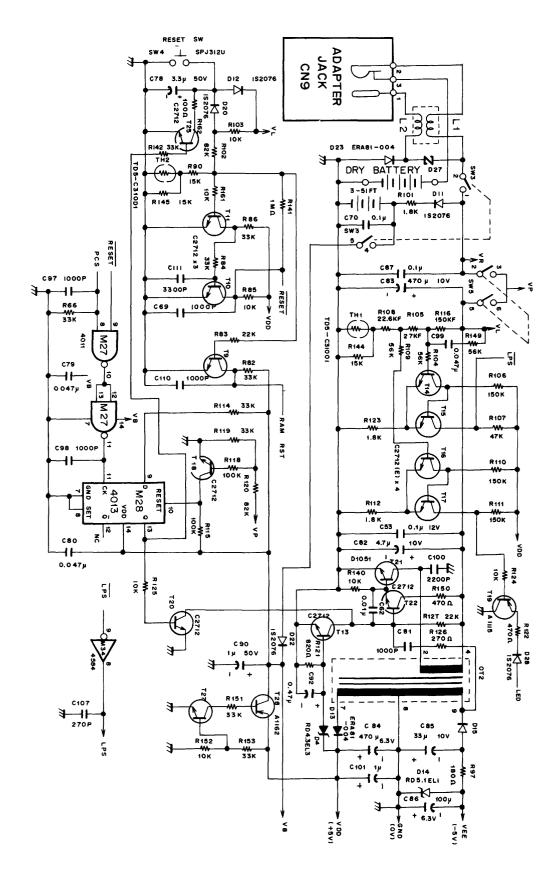
Figure 4-25. Power Supply and Reset Circuit
