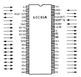
Figure C-2. Pin Configuration of 80C85A
