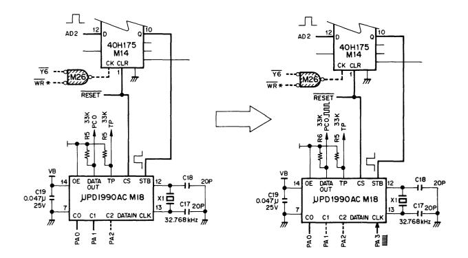
Figure 4-13. Time Read Sequence of  $\mu$ PD1990AC
