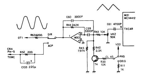
Figure 4-18. Transmission Filter Circuit
