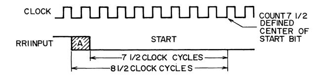
Figure C-15. Start Bit Detection Timing
