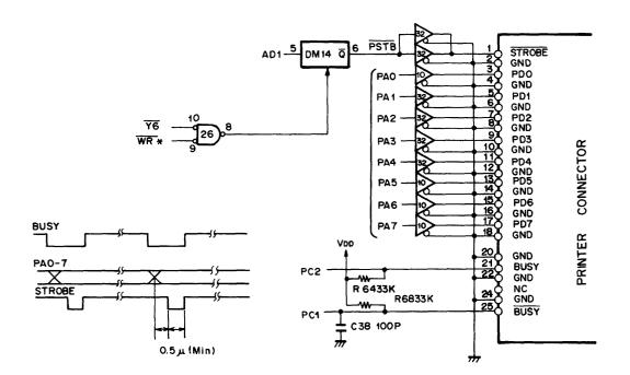
Figure 4-9. Printer Interface Circuit
