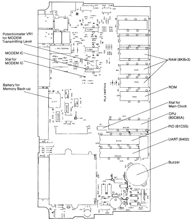
Figure 1-4. Main PCB (Bottom View)
