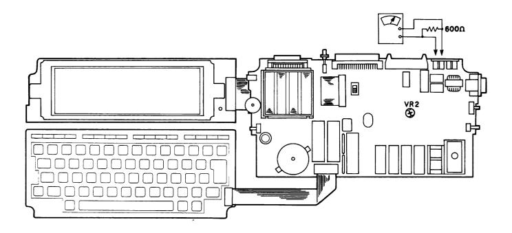
Figure 4-20. MODEM Adjustment
