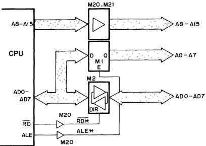
Figure 4-3. Functional Block Diagram of Bus Separation Circuit
