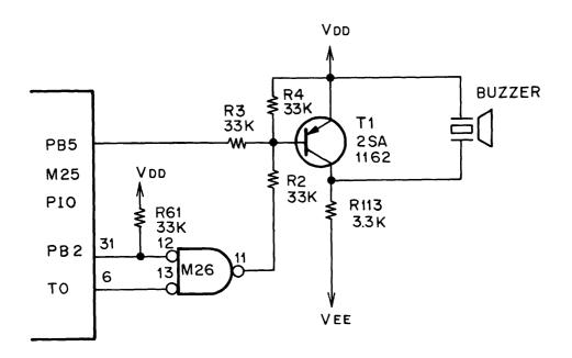
Figure 4-11. Buzzer Control Circuit
