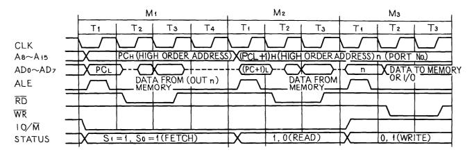
Figure C-4. 80C85A Basic System Timing
