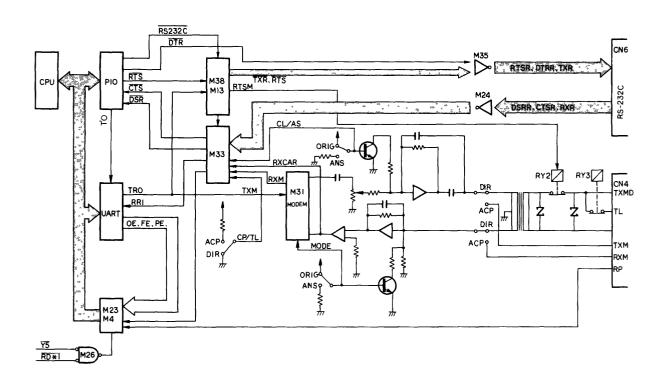
Figure 4-14. Functional Block Diagram of the Serial Interface
