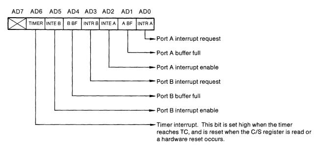
Figure C-9. Reading the C/S Register
