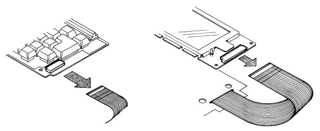
Figure 2-2. Keyboard and LCD PCBs Removal
