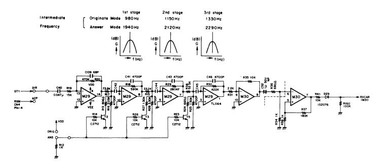
Figure 4-19. Reception Filter Circuit
