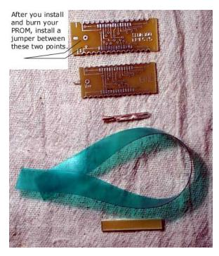
In the photo at the left (from top to bottom) you see the raw MOMBO board, followed by a "trimmed" MOMBO board, some jumper stock, a strip of extraction ribbon—used to remove a MOMBO from the Molex socket in a Model 100, 102 or 200, and a stand-off/spacer.
