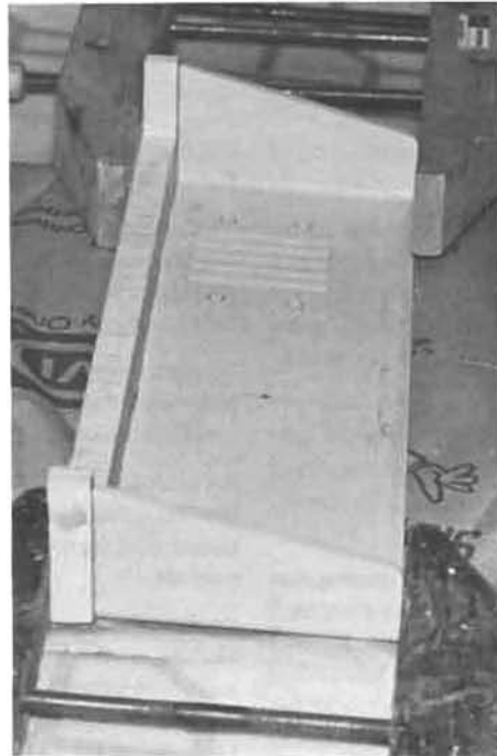
Photo 5. View of the keyboard base before final trimming. The three pieces of wood were installed one at a time allowing time for the glue to cure.
