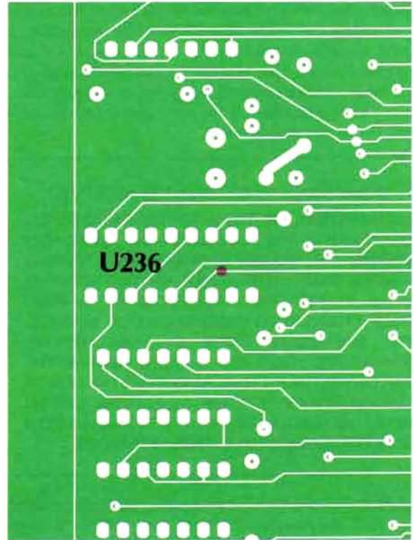
Figure 3. Trace cut at U236 on the foil side of the board.
