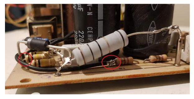
O Install a **1N5408** diode between **R1**(lead far from AC-In (J3)) and **HV-Ground**, with stripe facing R1.
