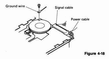
2. A power supply cable for an additional FDD is already prepared on the mounting bracket of the FDD. Remove it from the bracket by removing the nylon binder.
