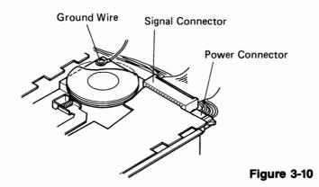
1. Disconnect the signal and power cables from the FDD (Floppy Disk Drive). On the body of the A-drive FDD, the ground wire is secured. Disconnect it by removing the screw.
