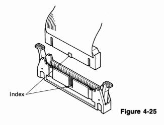
12. Connect the signal cables and power cables to both FDDs.
