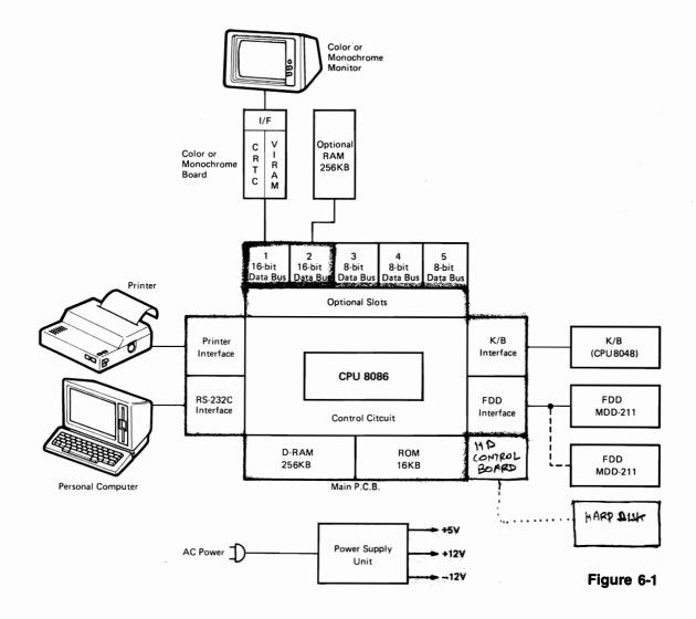
The main P.C.B. consists of the 8086 16-bit microprocessor, 256K bytes of system RAM, 16Kbyte ROM which contains the power-on diagnostic program, BIOS and IPL (initial program loader), the printer interface, asynchronous communication interface, keyboard interface, floppy disk drive interface. Another various control circuits are also equipped with the computer in order to work these elements effectively.
