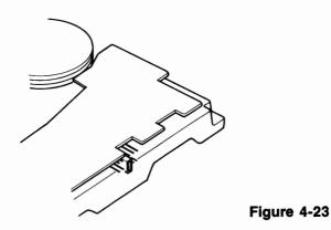
8. Turn the mounting bracket upside down and secure the optional FDD with four screws.
