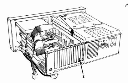
Before removing the Color/Graphics Monitor Adapter in expansion slot 1, disconnect the 3-pin connector that comes from the display as shown in the figure below.
