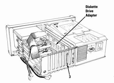
Connect the signal cable connector with two groups of wires on the bottom diskette drive, then connect the remaining connector to the top diskette drive as shown below.
