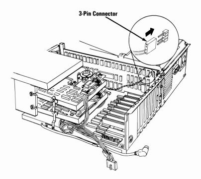
If you removed an option from slot number 2, install the option by holding the top corners and firmly press the option into the expansion slot. If this option is as long as the Color/Graphics Monitor Adapter just installed, make sure the front of the option is seated in the card support bracket on the front panel.
