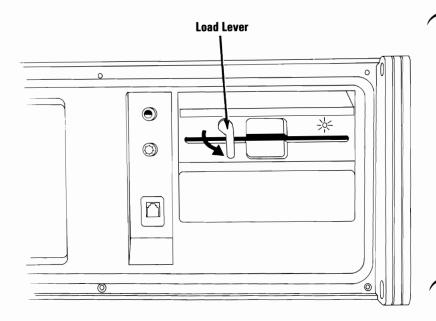
When the system is using the diskette drive, the In-Use light on the front of the drive will be on. To remove a diskette from the drive, rotate the load lever clockwise and pull out the diskette.
