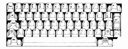
Key positions in the typewriter area are much like those of a standard typewriter. There are, however, some additional keys that perform control functions for the IBM Portable Personal Computer.
