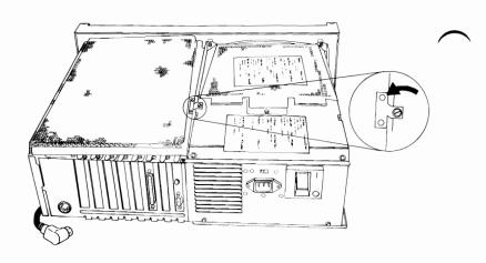
16 Carefully lift the shield from the system unit. Set the shield aside.
