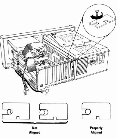
Install the shield by placing the notches over the guides in the front panel, then lower the shield.
