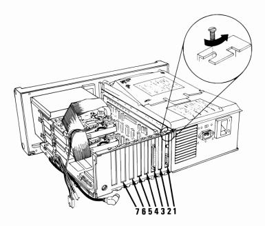
29 If you have an option installed in expansion slots 4 through 7, grasp the option by the top corners and pull straight up until it is loose from the expansion slot. Set the option aside.
