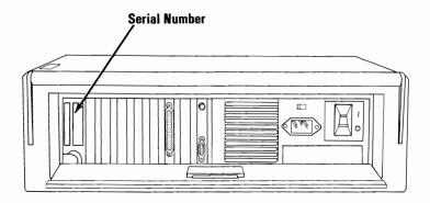
6 Set the input-voltage selector switch to match your power source (115 or 230 Vac).
