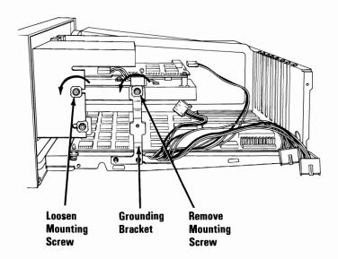
39 Loosen the mounting screw to the front-panel face plate with a 5.5-mm (7/32-in.) open-ended wrench or a 3-mm allen wrench.
