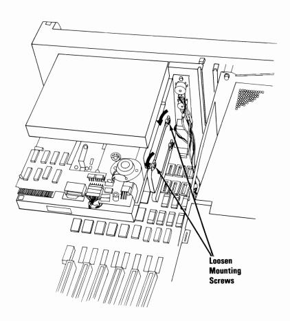
41 Loosen the mounting screw to the front-panel face plate with a 5.5-mm (7/32-in.) open-ended wrench or a 3-mm allen wrench.
