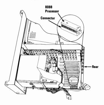
25 Carefully insert the module puller between one end of the 8088 and its connector as shown below. Rock the module puller from side to side until the end of the 8088 raises slightly. Repeat this procedure at alternate ends until the 8088 is free of the connector. Remove the 8088 from the system board and set it aside.
