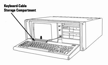
Pivot the keyboard up. Press the two keyboard release latches toward the center of the system while pushing the keyboard against the front panel. Release the latches.
