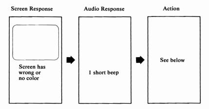
If you are using a TV as your display, verify that the color is correct by disconnecting your TV from the unit. Operate your TV normally to verify color quality. Also ensure your TV is compatible with U.S. Television Broadcast Standard. If you have an IBM Color Display, go to Test 9000.
