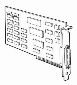
This option consists of the Synchronous Data Link Control (SDLC) Communications Adapter. If it is missing or damaged, notify your place of purchase.
