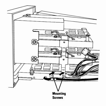
Insert the diskette drive mounting screws into the right diskette drive mounting holes. Do not tighten.
