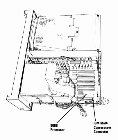
Compare your coprocessor with the one in the figure below. Find the notch in your coprocessor safety protector shown in the figure. This notch must face the 8088 processor and be toward the rear of the system board. If this is not possible, the safety protector was not assembled correctly. Go back to step 19.
