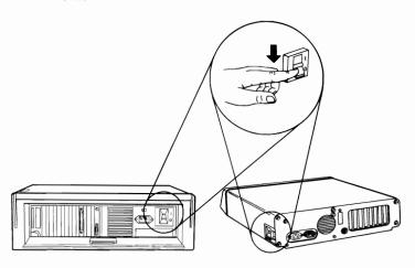
8 Unplug the system unit's and expansion unit's power cord from the wall outlet. Disconnect all cables and power cords from the rear of the units.
