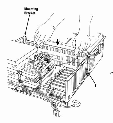
Connect the 3-pin connector from the display cable to the three pins at the rear of the option. As shown in the figure below.
