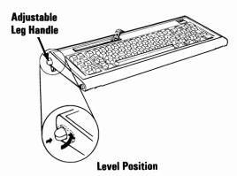
Press the adjustable leg handles in again and slide them into the bottom holes on the front panel.
