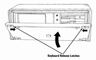
To lower the keyboard down to the operating position, press the two keyboard release latches toward the center of the system and lower the keyboard. Release the latches.
