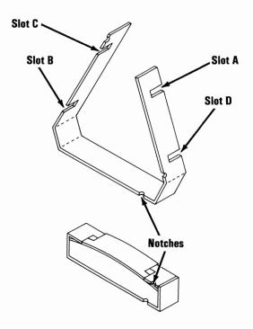
20 Install the safety protector on the coprocessor as shown below. Make sure the notch in the safety protector is on the same end as the notch in the coprocessor. The overlapped portions of the safety protector should be on the bottom or pin side of the coprocessor.
