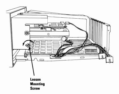
Place the system unit so the rear faces you. Use a 5.5-mm (7/32-in.) open-ended wrench or a 3-mm allen wrench to loosen the diskette drive mounting screws on the right side (Do not remove the screws from the threaded screw holes).
