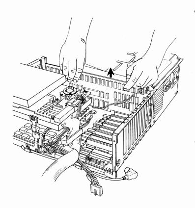
35 Disconnect and remove the signal cable from the back of your diskette drive. Set the cable aside.
