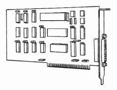
This option consists of the Binary Synchronous Communications Adapter. If it is missing or damaged, notify your place of purchase.
