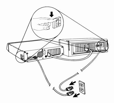
5 Check the wall outlet by plugging in a working lamp.
