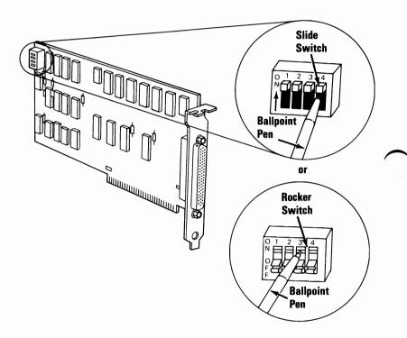
2 Switch settings on the Extender Card must reflect the total amount of memory on the system board. The following figure shows the setting for the amount of total memory. Set the switches on your Extender Card now.
