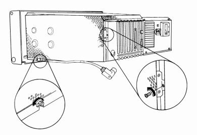
Place the system unit so the rear faces you. Remove the third mounting screw on the shield as shown below.
