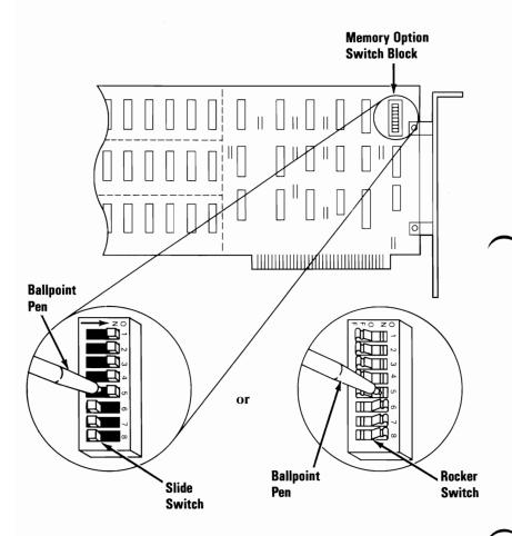
5 Switch settings on the 64/256KB Memory Expansion Option indicate the total amount of memory on the system board and the Memory Expansion Option. The following figures show the settings for the various amounts of total memory. Set the switches on your 64/256KB Memory Expansion Option now.
