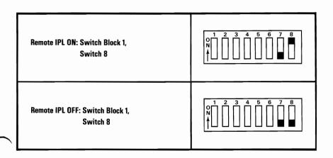
Fill in the necessary information for the adapter number, station address, and remote IPL in step 4 of the "Test 2200" section. The IBM Cluster Adapter can be installed in your system unit or your expansion unit. If your are installing this option in your IBM Portable Personal Computer, it can only be installed in expansion slot 2.
