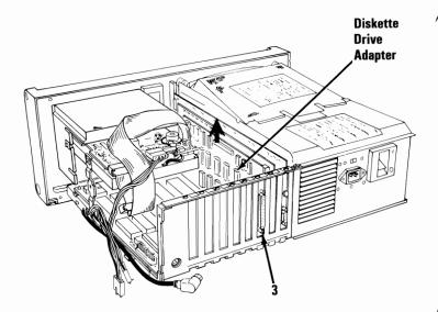
Disconnect the Diskette Drive Signal Cable from the front of the adapter. Set the Diskette Drive Adapter aside.
