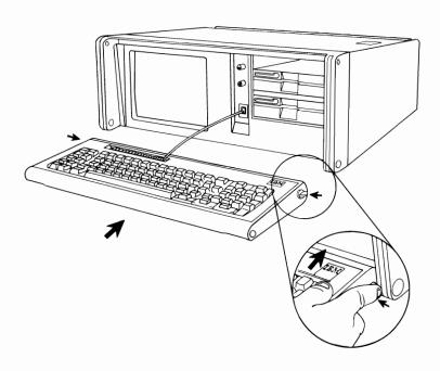
8 If the keyboard cable is extended, store the coiled portion of the cable in the keyboard-cable storage compartment.
