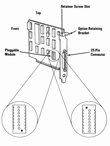
Module Position for Current-Loop Interface Module Position for RS232-C Interface Note: There is a small black jumper included with this option in its own plastic bag. This jumper will not be used with your IBM Portable Personal Computer.
