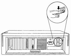
3 Unplug the system unit's power cord from the wall outlet. (If the expansion unit is attached, unplug its power cord also.) Disconnect all cables and the power cord from the rear of the system unit.
