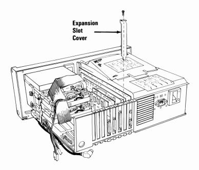
Hold the option by the top corners and firmly press it into expansion slot 2, 4, 5, 6, or 7.
