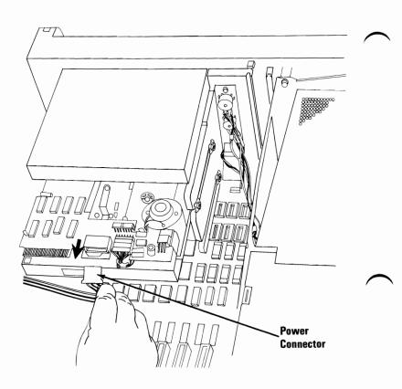
Place your system unit so that the right side faces you. Use a flat-blade screwdriver or a 5.5-mm (7/32-in.) open-ended wrench and remove the two mounting screws that hold the diskette drive grounding bracket.
