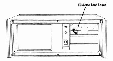
Remove the shipping cardboard. If you have two diskette drives installed in your system unit remove the shipping cardboard from both drives.
