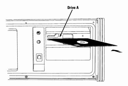
2 Close the diskette drive by rotating the load lever counterclockwise.
