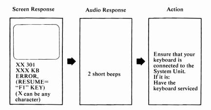
Note: Ensure the keyboard is connected correctly and check for any objects or foreign material on the keyboard. If after having the keyboard serviced, error 301 still appears, have the system unit serviced.
