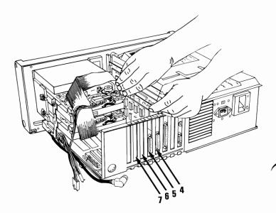
For each of the adapters just installed in the expansion slots, align the slots in the adapter retaining brackets with the hole in the rear panel of the system unit. Insert the screw and tighten with a flat-blade screwdriver or a 5.5-mm (7/32-in.) open-ended wrench.
