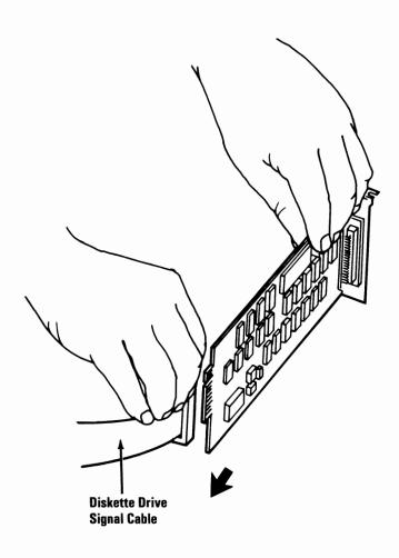
32 If you have an option installed in expansion slot number 2, grasp the option by the top corners and pull straight up until it is loose from the expansion slot. Set the option aside.
