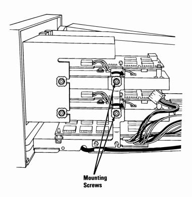
Align the diskette drives so they are flush (tight against) with the front panel. Use a flat-blade screwdriver, 5.5-mm (7/32-in.) open-ended wrench or a 3-mm allen wrench to tighten the diskette drive mounting screws and two diskette drive grounding bracket screws.
