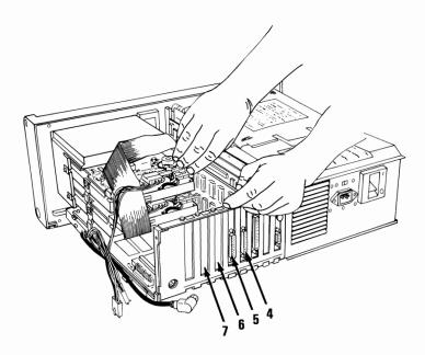
30 Grasp the Diskette Drive Adapter in expansion slot 3 by the top corners and pull straight up until it is loose from the expansion slot.
