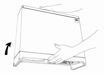
11 Slide the system-unit cover up until it clears the frame of the system unit. Set the cover aside.
