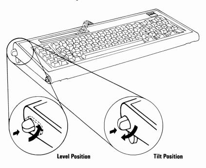
To attach the keyboard to the front panel press the adjustable leg handles in and slide them into the bottom holes on the system unit's front panel.
