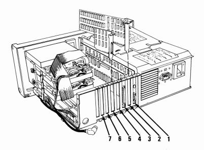
Some options come with instructions to install a card support bracket in your system unit. The IBM Portable Personal Computer has a card support bracket already installed, so discard the bracket packaged with the option. Continue with the next step.
