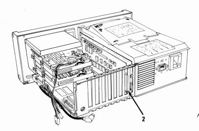
57 Connect the Diskette Drive Signal Cable to the front end of your Diskette Drive Adapter as shown below.
