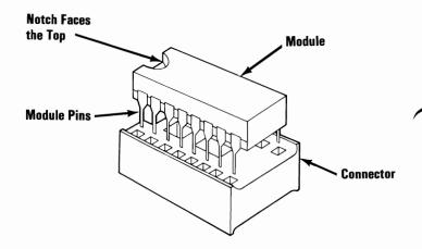
3 Check to see that all of the pins on each module are seated properly in the connectors and that all the notches are facing the top of the option. If the modules are incorrectly installed, you can remove the modules with a module puller, as shown below.
