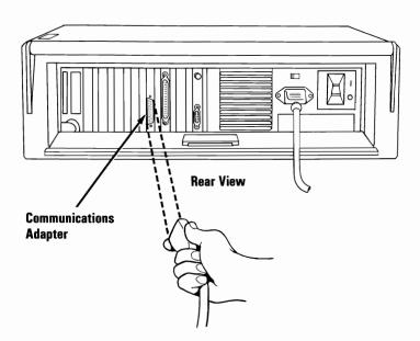
6 Connect the other end of the Communications Adapter Cable as shown in the example, and tighten the screws clockwise.
