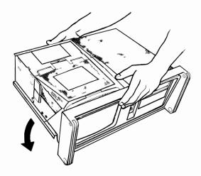
Place the system unit so the right side faces you. Disconnect the internal keyboard-cable connector, as shown below.
