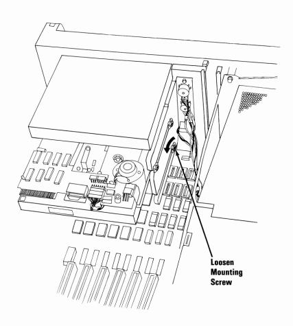
42 Slide the diskette drive out of its mounting bracket by sliding it to the rear. Set the diskette drive aside.
