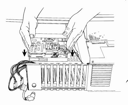
43 Study the figure below and note the location of the terminating resistor on the diskette drive you just removed (drive A). Make sure this diskette drive with the terminating resistor is installed in the top position. Ensure that the lower diskette drive (drive B) does not have the terminating resistor installed.
