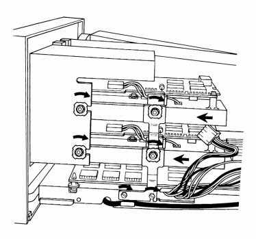
Place the system unit so the rear faces you. Use a 5.5-mm (7/32-in.) open-ended wrench or a 3-mm allen wrench to tighten the screws mounted on the right side of the diskette drives.
