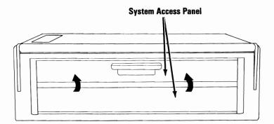
If the keyboard is separated from the front panel, press in firmly on the adjustable leg handles of the keyboard and place the legs in the closed position as shown.
