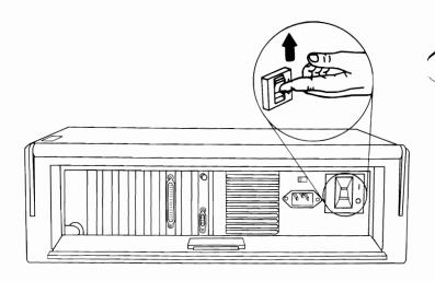
To operate the system unit, you simply set the Power switch to On. Your commands to the system can then be entered through the keyboard. You will see your commands and the system responses on your display. If a printer is attached to your system unit, you may also request a printed copy of almost any data in the system.
