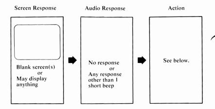
Note: Ensure that your input-voltage selector switch on your system unit is set correctly.
