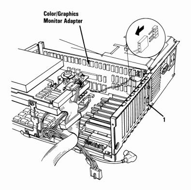
34 Grasp the Color/Graphics Monitor Adapter by the top corners and pull straight up until it is loose from the expansion slot. Set the adapter aside.
