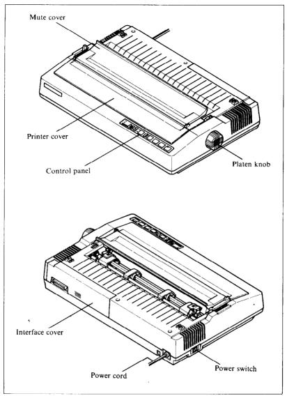
Figure 2-1. Front and rear views of the printer.
