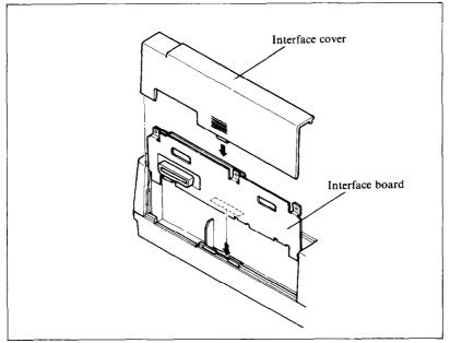
Figure 1-7. Slide the I/F board into the slot.
