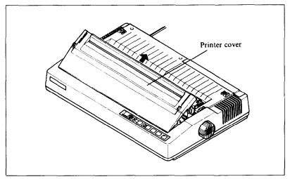
Figure 1-2. Remove the printer cover by lifting carefully.
