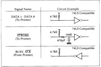
Figure F-2. Typical interface circuit.
