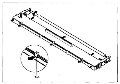
Figure 8-1. Unhook tabs to open the cartridge.
