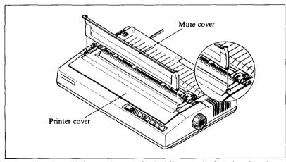
Figure 1-6. Install the mute cover by holding vertically, then lay down on the printer cover.
