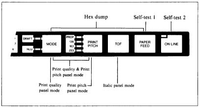
Figure 2-3. Extra functions while turning on the printer.
