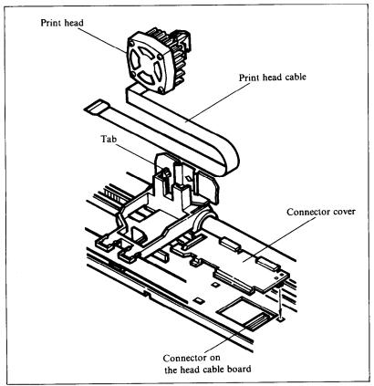
Figure 8-4. Replacement of the print head
