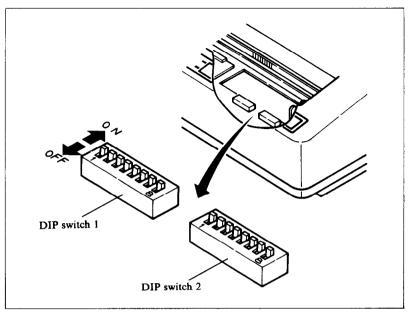
Figure A-1. The DIP switches are located under the printer cover.
