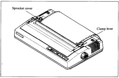
Figure 2-9. Open the sprocket covers to expose the sprocket teeth.
