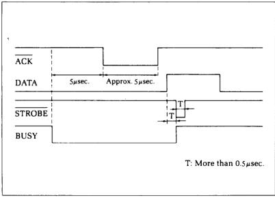
Figure F-1. The interface timing diagram.
