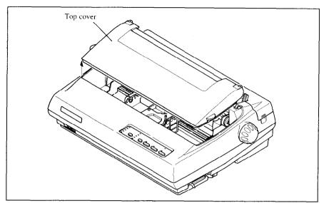
Figure 1-4. Removing the top cover
