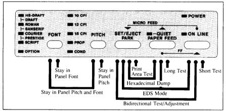
Figure 2-2. Power-up functions of control panel
