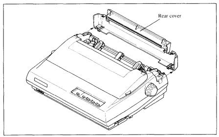
Figure 1-12. Removing the rear cover
