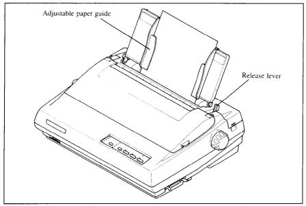
Figure 1-11. Loading a single sheet
