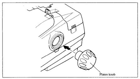
Figure 1-3. Mounting the platen knob
