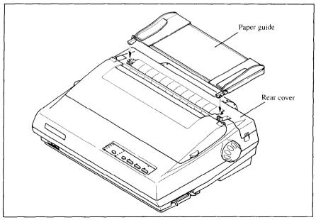
Figure 1-15. Mounting the paper guide for fanfold forms
