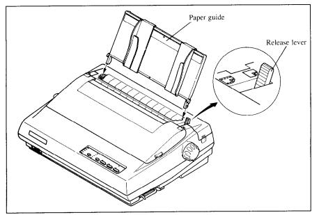
Figure 1-10. Mounting the paper guide for single sheets
