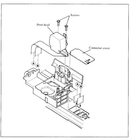
Figure 7-1. Replacing the print head
