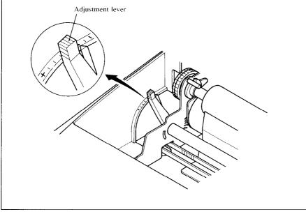
Figure 1-18. Location of the adjustment lever
