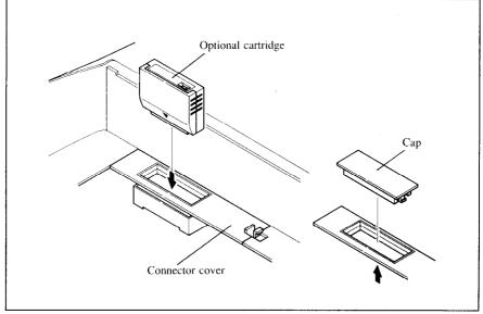
Figure 1-8. Slide the cartridge into the slot with the power switch off.
