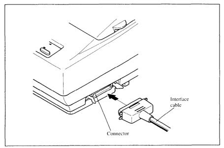
Figure 1-9. Connecting the interface cable
