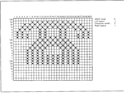
Figure 5-2. Telephone symbol with normal LQ pica
