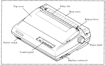
Figure 1-2. The printer's external parts
