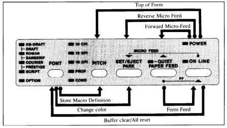
Figure 2-7. Switch combination functions of control panel
