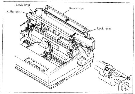
Figure 1-7. Install the roller unit onto the printer
