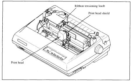
Figure 1-5. Installing the ribbon cartridge
