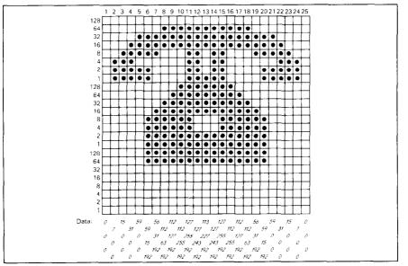
Figure 5-5. Compressed character pattern of telephone symbol
