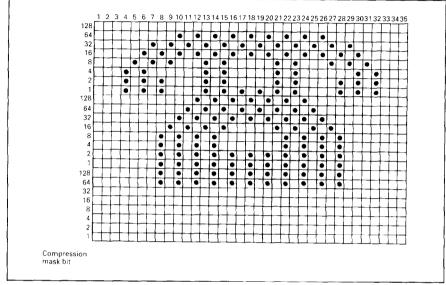
Figure 5-3. Telephone symbol with LQ pica
