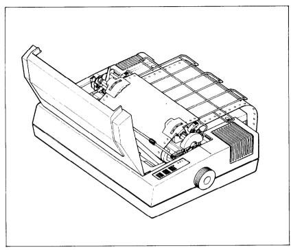
Figure 2-8. SD-10/15 ready to run with sprocket-feed paper.
