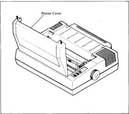
Figure 1-2. Remove the printer cover by lifting straight up.
