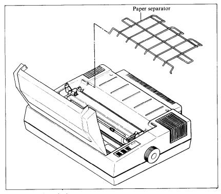
Figure 1-6. Attach the paper separator.
