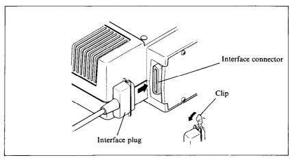
Figure 3-1. SD-10/15 has parallel interface as standard.
