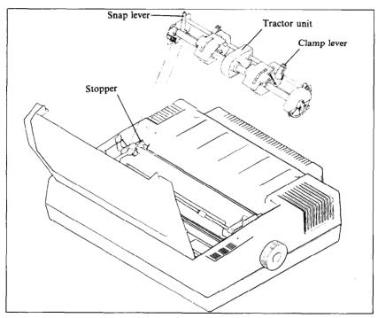
Figure 2-6. Replace the tractor unit by placing the hooks against the stoppers and lower the front into place while holding the snap levers.
