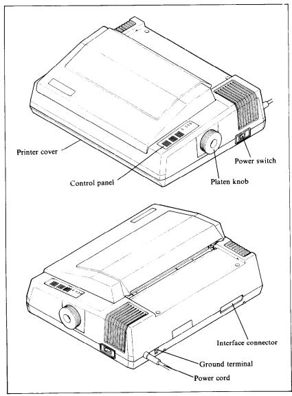
Figure 2-1. Front and rear views of SG-10.
