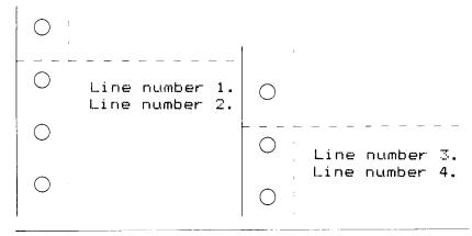
The form feed (CHR\$(12)) in line 50 caused the printer to move to the top of a new page before printing the last two lines.
