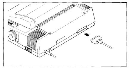
Figure 3-1. SG-10/15 has parallel interface as standard.
