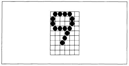
Figure 9-3. Dots can be inside boxes or straddle the vertical lines of the grid.
