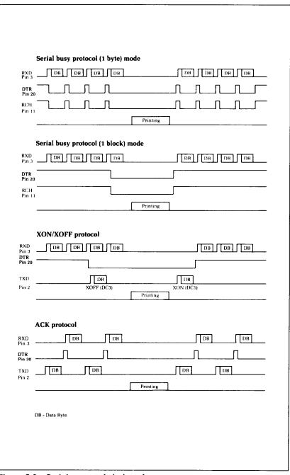
Figure I-2. Serial protocol timing charts.
