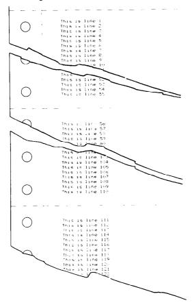
Always send a form feed after setting the top margin, or it will not work on the first page printed. That's because the top margin only takes effect after a form feed.
