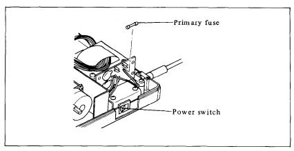
**Figure 11-1.** After removing the screws, pull the upper case slightly forward and lift it off the printer. The fuse is located near the power switch.
