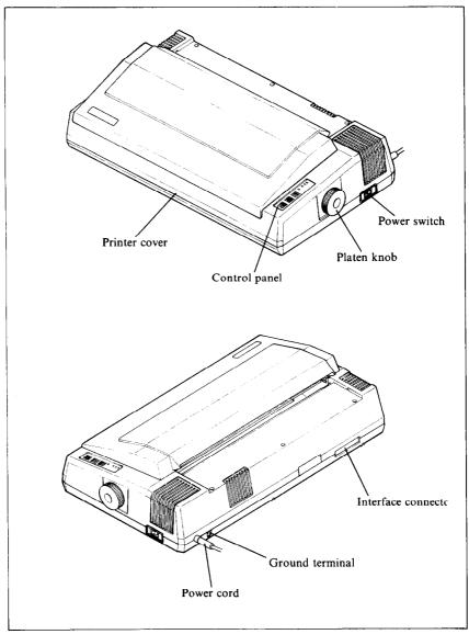
Figure 2-2. Front and rear views of SG-15.
