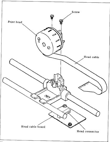
Figure 11-2. Replacement of SG-10/15's print head is simple.
