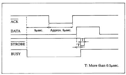
Figure H-1. SG-10/15 interface timing diagram.
