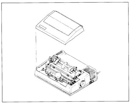
Figure 1-2. Remove the printer cover by lifting carefully.
