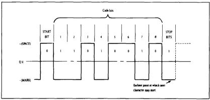
Figure I-1. Typical data byte on the serial interface.
