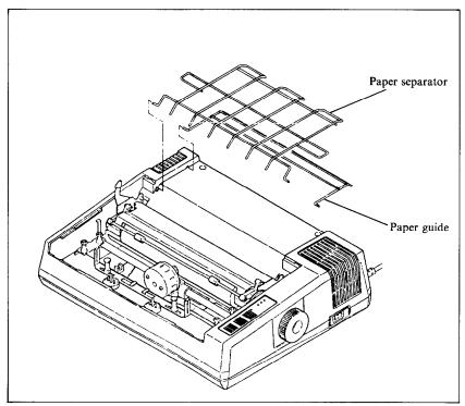
Figure 1-6. Attach the paper separator and paper guide.
