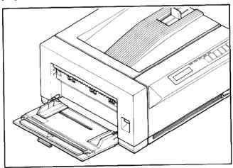
3. Press the release button (at the right) upwards and open the cover.
