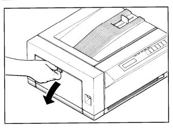
2. Hold the arrow at the center of the multi-purpose tray, then pull out the extension tray.
