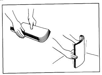
5. Align the right side of the stack of paper with the right-hand paper guide. Slide the paper stack gently into the printer as far as it will go. Make sure that the height of the paper stack does not exceed the mark on the paper guide.
