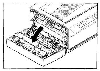
2) Remove the EP-L cartridge by pulling the tab.
