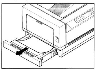
6) If paper is jammed in the fixing assembly area, pull the paper back into the printer and remove it.
