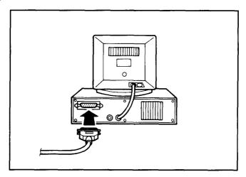
**NOTE**: The printer's factory setting is for a parallel interface. If the other interface is to be used, you need to select the interface on the control panel. See "4.3.1 Selecting the Interface" for selecting the type of interface.
