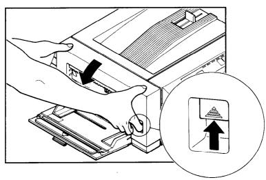
4) If you have been printing with the multi-purpose tray, check the paper pick-up area first. If there is a paper jam here, remove the paper by pulling it in the direction of the arrow.
