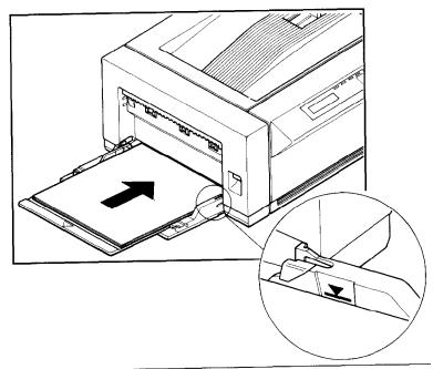
6. Slide the left-hand paper guide so that it touches the left side of the paper stack. Make sure that the paper guide does not press too tightly or fit too loosely against the paper stack. Otherwise, this can cause paper jams or other problems.
