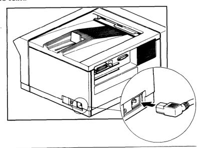
Only use the power cable supplied with the printer. Note that this power cable is fitted with a ground pin. This grounding is an important safety feature and should not be ignored. If a suitable grounded socket is not available, contact a qualified electrician to rectify the situation.
