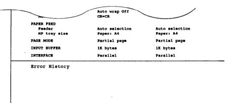
This means that the Centronics parallel interface is active. If the serial port were active, that line would state serial.
