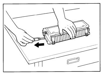
Make sure that the tab is pulled smoothly in a direction parallel to the flat surface. Otherwise, the tape may break or snap, making the cartridge unusable.
