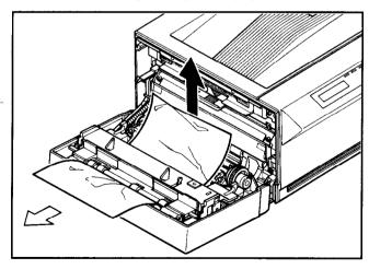
8) If the paper has passed completely through the fixing assembly area, pull it out in the direction of the arrow.
