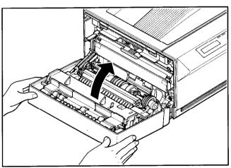
2. Lift the multi-purpose tray and close it until it latches on both sides.
