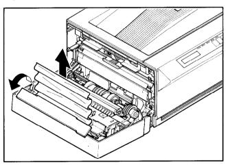
10) After checking all the areas described here, close the side cover, replace the face-up tray (if it is being used), pull out the extension tray and refill the multi-purpose tray. Printing will restart.
