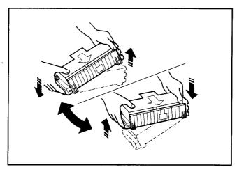
5. Place the cartridge on a flat surface. While holding down the cartridge with one hand, use the other hand to pull the orange tab to remove the seal.
