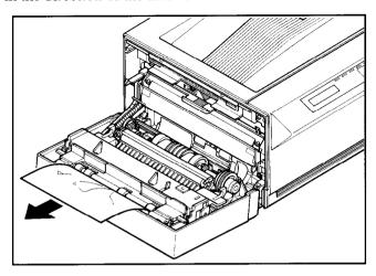
9) If a paper jam has occurred in the face-up delivery area, put the paper straight upwards to remove it.
