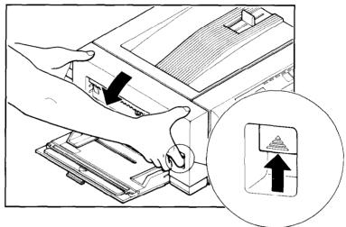
3. To increase print density, move the density adjustment lever to the right. To reduce the density, move the lever to the left.
