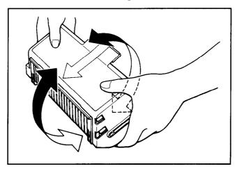
4) Replace the EP-L cartridge in the printer, then close the side cover.
