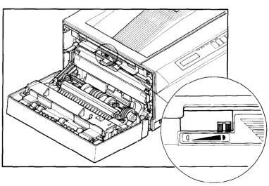
**NOTE**: The density adjustment lever has four settings from left to right. As you move the lever, it clicks at each of the two positions in the middle.
