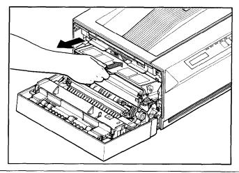
3) Hold the EP-L cartridge as shown below, then rock it gently back and forth about 45 degrees in each direction, about 5 or 6 times. This will redistribute the toner inside the cartridge.
