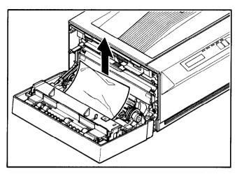
7) If the paper does not extend from the side of the fixing assembly area, pull it in the direction of the black arrow. If the paper is extracted in the opposite direction, infused toner can be deposited inside the printer, staining the back of subsequently printed pages.
