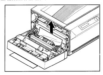
**CAUTION:** The fixing assembly area becomes extremely hot when the printer has been operated for some time. Never touch this area when the printer is open. Otherwise, personal injury may result.
