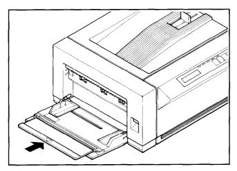
2) If the face-up tray is installed, remove it.
