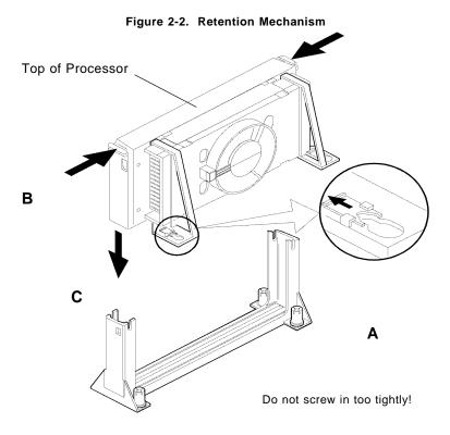
6. Slide the clips on the supports (A) forward until they click into place to hold the pegs securely. Apply slight pressure on the peg and push the peg toward the clip while pushing the clip forward. Push the latches on the processor (B) outward until they click into place in the retention mechanism. The latches must be secured for the proper electrical connection of the processor.
