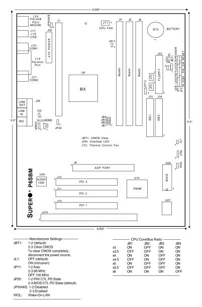
Note: There are two CD connectors of different sizes. Use only the one that matches the size of the connector from your CD player. The MPEG connector is for use with a DVD decoder card.
