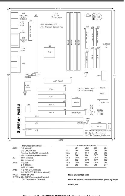
Figure 1-8. SUPER P6SBU Motherboard Layout
