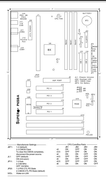
Figure 1-12. SUPER P6SBA Motherboard Layout
