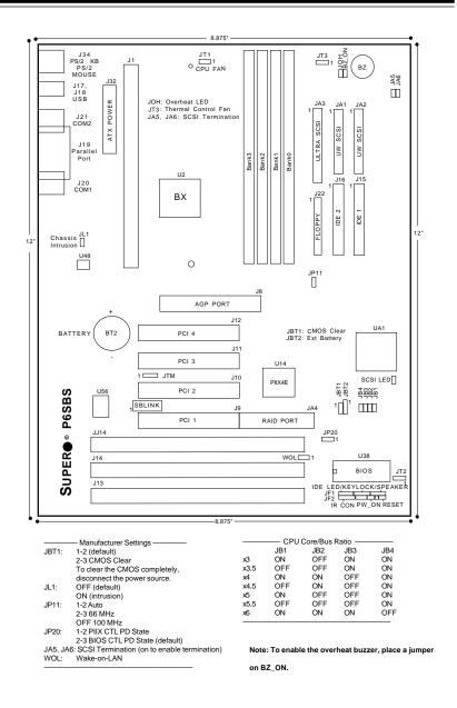
Figure 1-10. SUPER P6SBS Motherboard Layout
