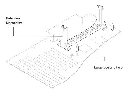
Figure 2-1. Mounting the Pegs
