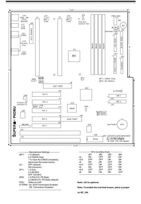
Figure 1-6. SUPER P6DBU Motherboard Layout
