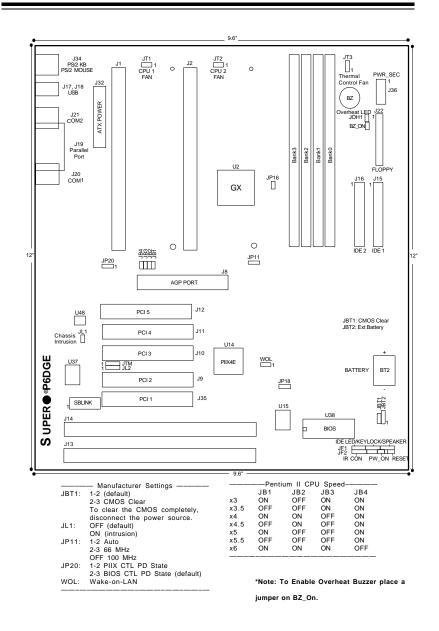
Figure 1-6. SUPER P6DGE Motherboard Layout
