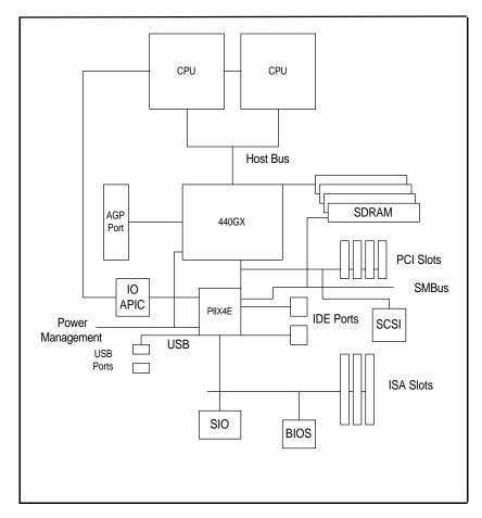
Figure 1-9. 440GX AGP SET: System Block Diagram (Dual Processors)
