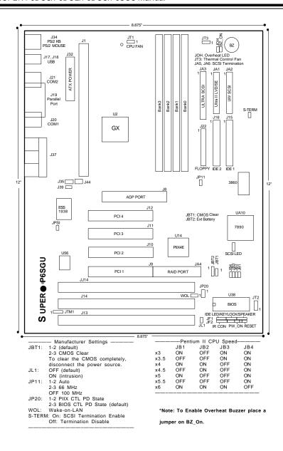
Figure 1-8. SUPER P6SGU Motherboard Layout
