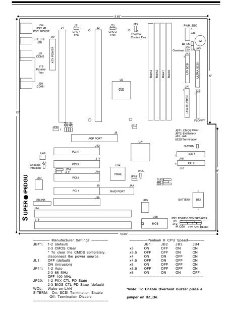
Figure 1-7. SUPER P6DGU Motherboard Layout
