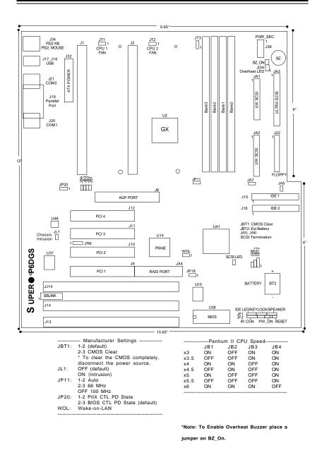
Figure 1-5. SUPER P6DGS Motherboard Layout
