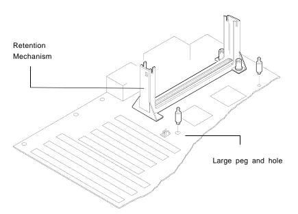
Figure 2-1. Mounting the Pegs
