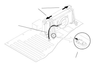
Figure 2-3. Attaching the Fan Power Cable
