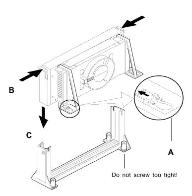
Figure 2-3. Retention Mechanism
