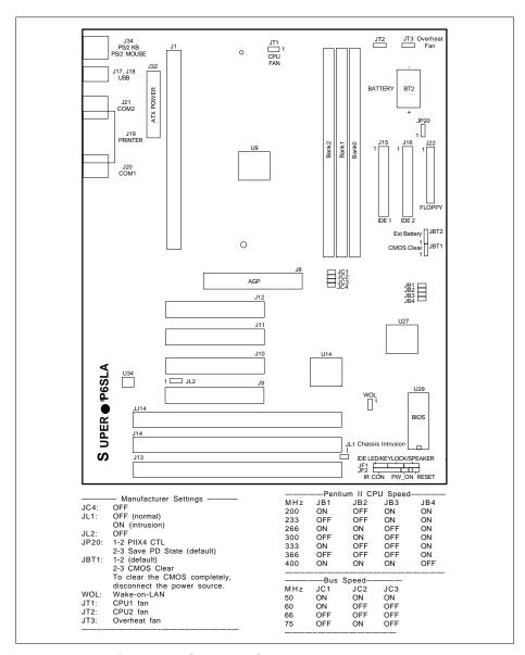
Figure 1-7. SUPER P6SLA Motherboard Layout
