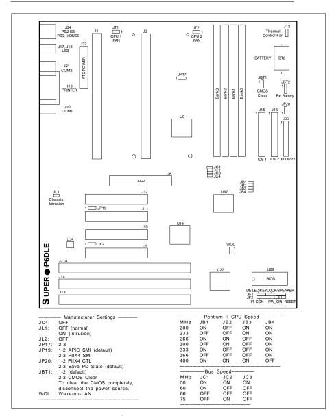
Figure 1-5. SUPER P6DLE Motherboard Layout
