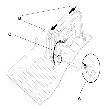
Figure 2-4. Attaching the Power Cable
