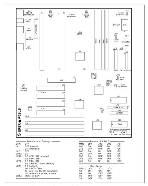
Figure 1-6. SUPER P6SLS Motherboard Layout
