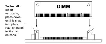
Figure 2-7. Installing/Removing a DIMM Memory Module
