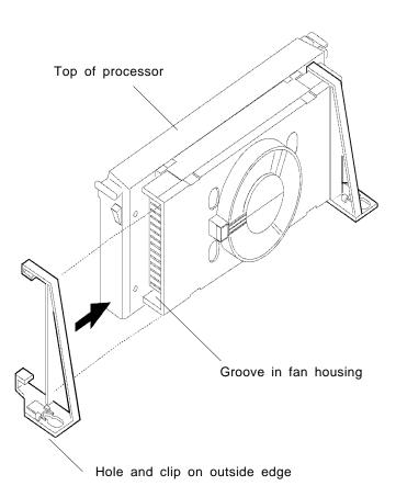
Figure 2-2. Support for Fan Heatsink
