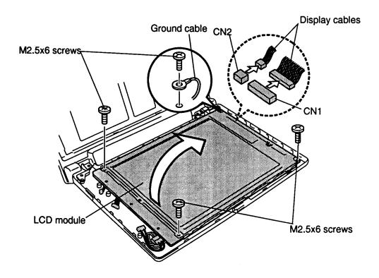
Figure 4-23 Removing the T2100 LCD module
