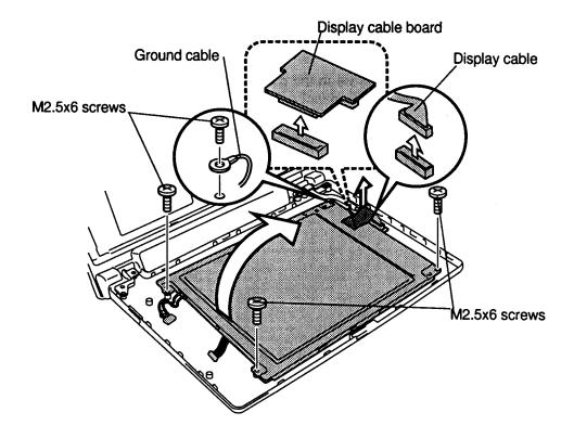
Figure 4-31 Removing the T2100CT LCD module and display cable board
