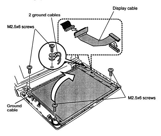
Figure 4-25 Removing the LCD module
