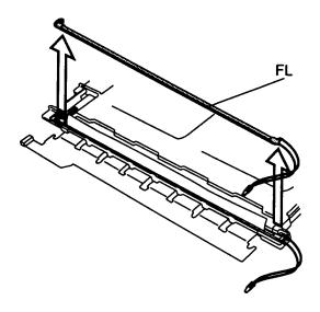
Figure 4-29 Lifting out the FL
