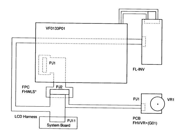
Figure 2-4 T2100CS display connection
