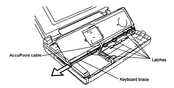
Figure 4-10 Removing the keyboard base
