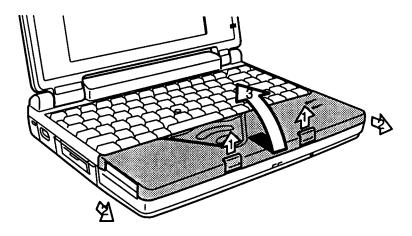
Figure 4-2 Unlatching the palm rest
