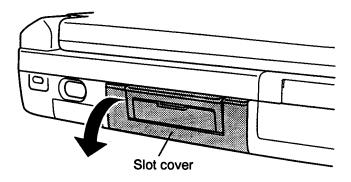
Figure 4-7 Opening the PCMCIA slot's cover
