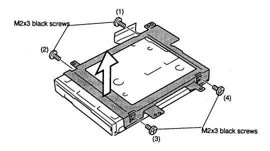
Figure 4-18 Removing the HDD
