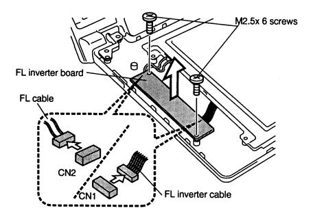
Figure 4-30 Disconnecting the FL inverter board
