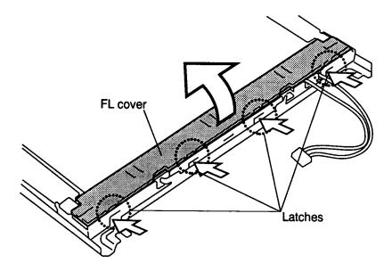
Figure 4-33 Removing the FL cover
