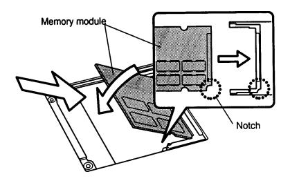
Figure 4-6 Inserting the memory module
