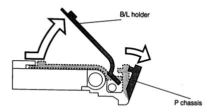
Figure 4-28 Removing the B/L holder
