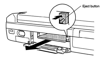
Figure 4-8 Removing the PCMCIA card
