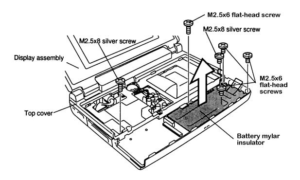
Figure 4-15 Removing the battery pack frame
