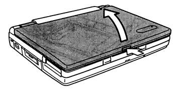
Figure 4-1 Opening the T2100 Series computer
