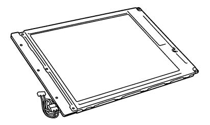
Figure 1-7 Monochrome LCD
