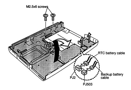
Figure 4-20 Removing the system board
