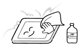
4. If water or other liquid is left on the panel's surface for a long period, it can change the screen's tint or stain it. Be sure to quickly wipe off any liquid.
