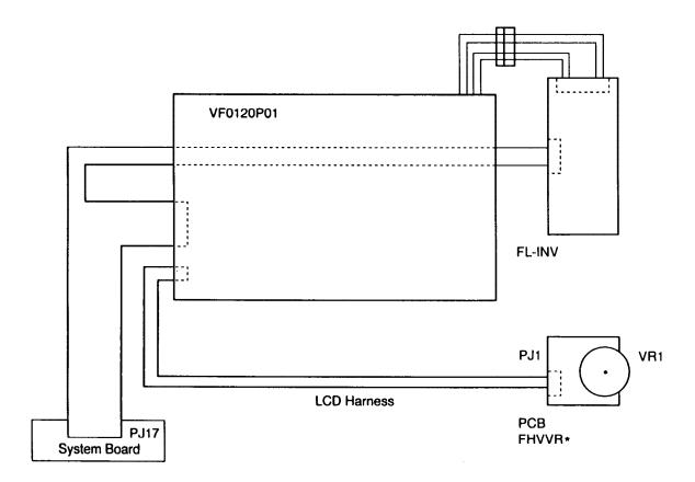
Figure 2-3 T2100 display connection
