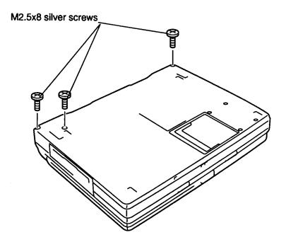
Figure 4-14 Removing the top cover screws
