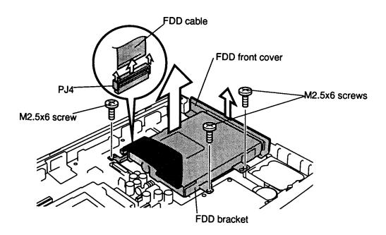
Figure 4-17 Removing the FDD with bracket
