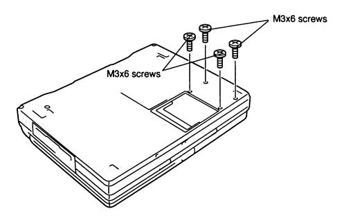
Figure 4-12 Removing the HDD screws
