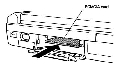
Figure 4-9 Installing an optional PCMCIA card
