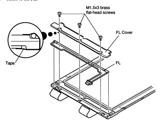
Figure 4-24 Removing the FL
