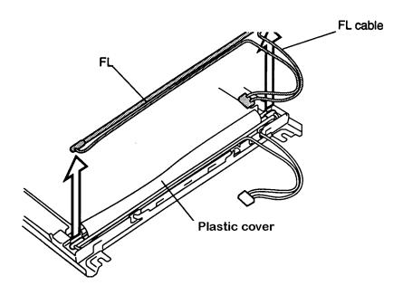
Figure 4-34 Removing the FL
