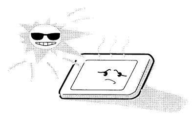
8. Do not store the module at temperatures below specifications. Cold can cause the liquid crystals to freeze, lose their elasticity or otherwise suffer damage.
