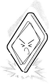
6. CMOS-LSI circuits are used in the module, so guard against damage from electrostatic discharge. Be sure to wear a wrist or ankle ground when handling the module.
