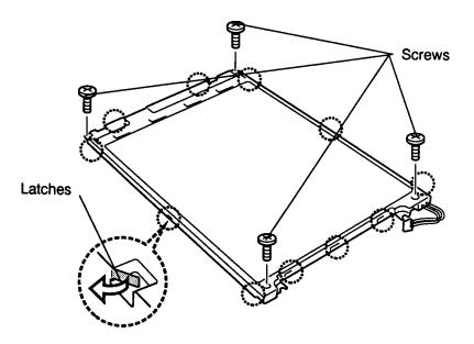
Figure 4-26 Unbending the color LCD module latches
