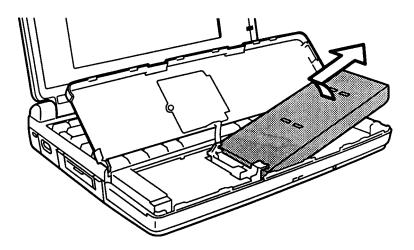
Figure 4-3 Removing the battery pack
