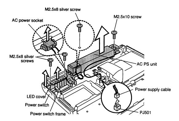
Figure 4-19 Removing the AC PS unit
