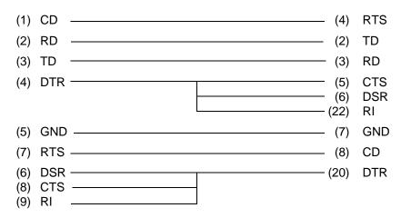
Figure G-4 RS-232-C direct cable (9-pin to 25-pin)
