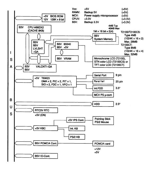
Figure 1-3 T2100/T2105 Series system board block diagram
