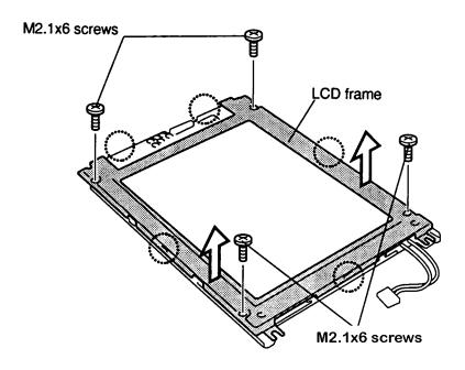
Figure 4-32 Removing the T2100CT LCD module screws
