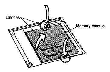
Figure 4-5 Removing the memory module
