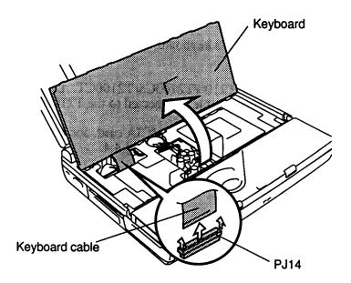
Figure 4-11 Removing the keyboard
