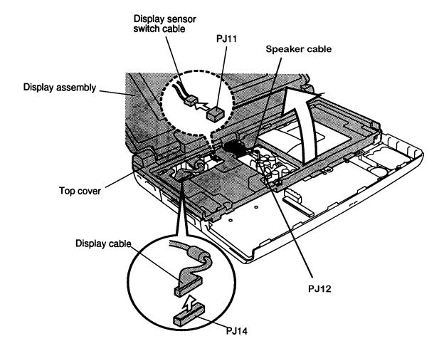
Figure 4-16 Removing the top cover & display assembly
