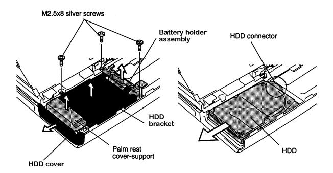
Figure 4-13 Removing the HDD
