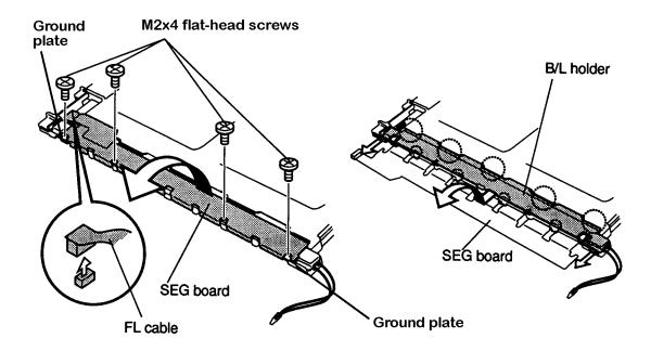
Figure 4-27 Removing the SEG board
