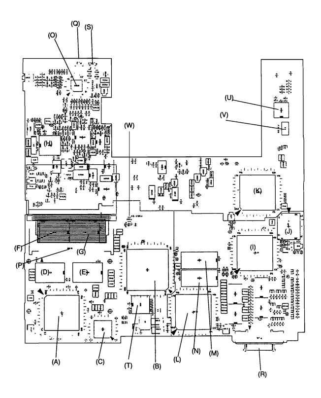
Figure B-2 FHVSY\* system board (back)
