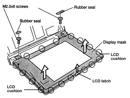
Figure 4-21 Removing the display mask
