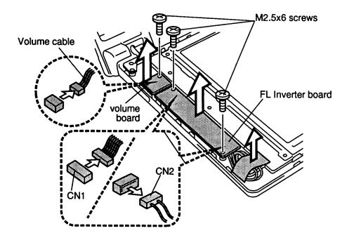
Figure 4-22 Removing the FL inverter and volume board
