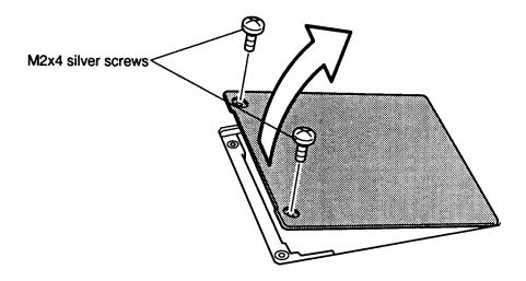
Figure 4-4 Removing the memory module socket cover
