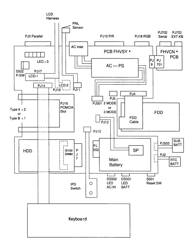
Figure 1-2 T2100/T2105 Series system unit configuration
