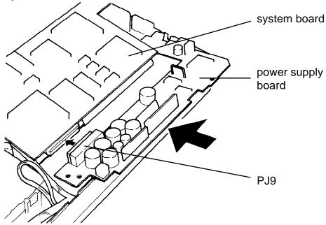
Figure 6-4 Positioning the power supply board
