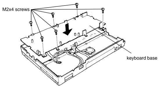
Figure 6-2 Securing the keyboard base
