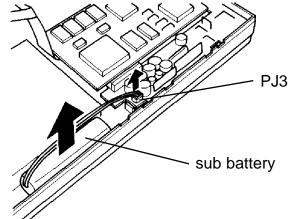
power supply board. Then remove the sub battery from the computer (Figure 5-14).
