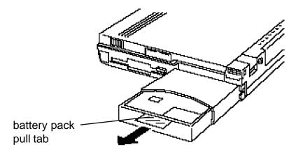
Figure 5-2 Removing the battery pack
