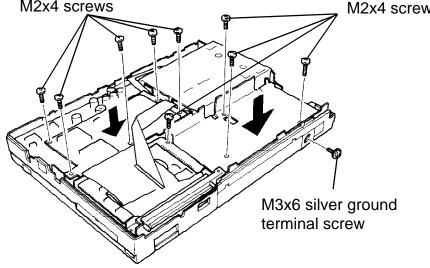
Figure 6-11 Installing the system board and middle base assembly screws
