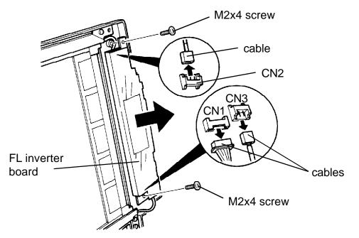
Figure 5-9 Removing the FL inverter board
