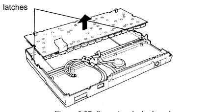
Figure 5-27 Removing the keyboard
