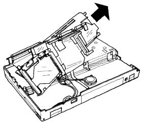
the flexible cables portion of the system board (Figure 5-18).
