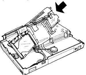
Figure 6-9 Routing the middle base assembly
