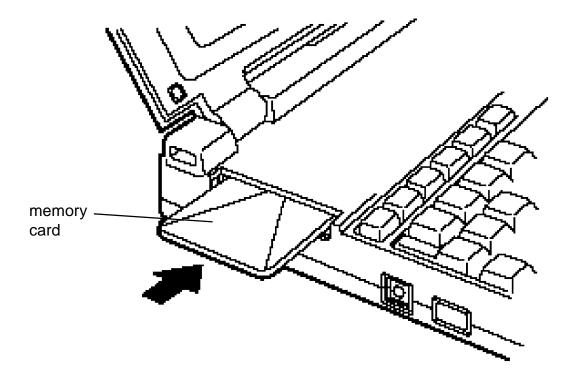
connection (Figure 6-22). DO NOT force the memory card into place. Figure 6-22 Inserting the optional memory card
