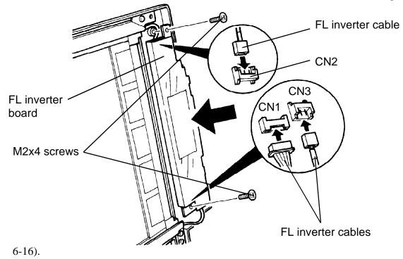
Figure 6-16 Installing the FL inverter board
