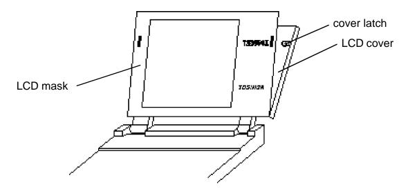
Figure 5-6 Releasing the LCD mask latches
