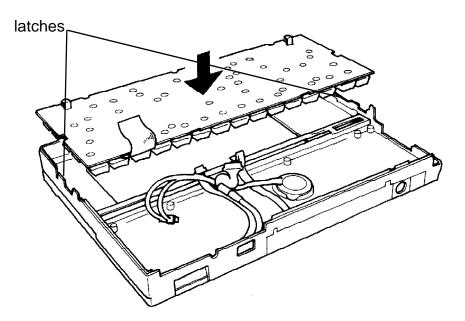
Figure 6-1 Installing the keyboard
