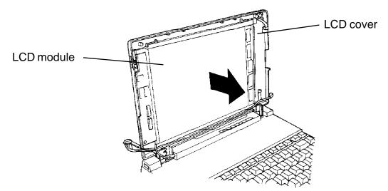
Figure 5-11 Removing the LCD module
