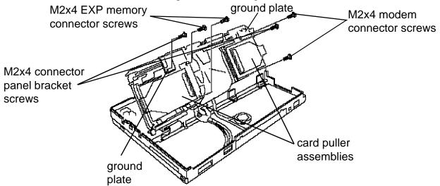
Figure 6-10 Installing the connector panel screws and ground plates
