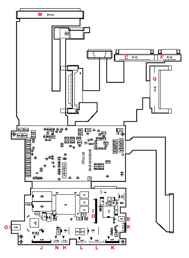
Figure A-3 System board FSTFGx (connectors) (front)
