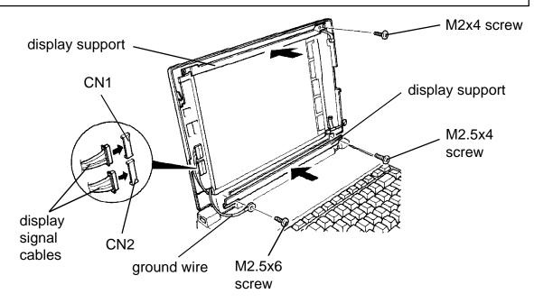
securing the LCD mask to the LCD cover. Figure 6-17 Installing the display supports and screws
