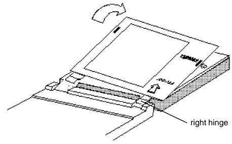
Figure 5-8 Removing the LCD mask
