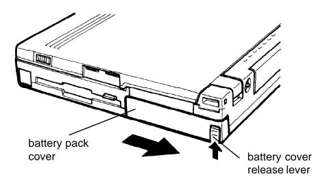
Figure 5-1 Removing the battery pack cover
