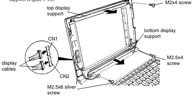
Figure 5-10 Removing the display supports
