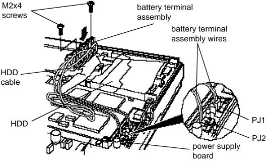
Figure 6-12 Installing the battery terminal assembly
