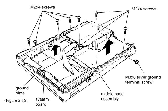
Figure 5-16 Removing the system board and middle base assembly screws
