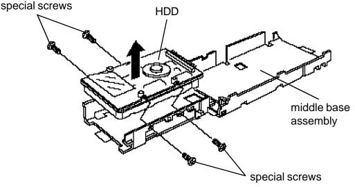
the HDD from the assembly (Figure 5-19).
