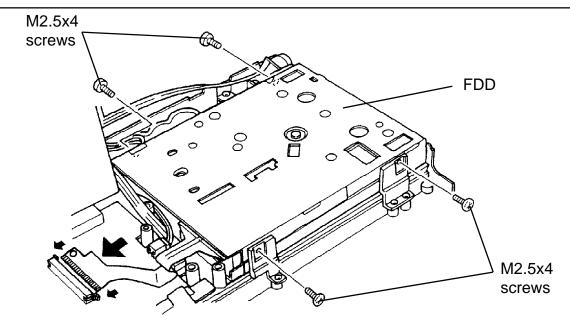
Figure 6-7 Securing the four FDD screws
