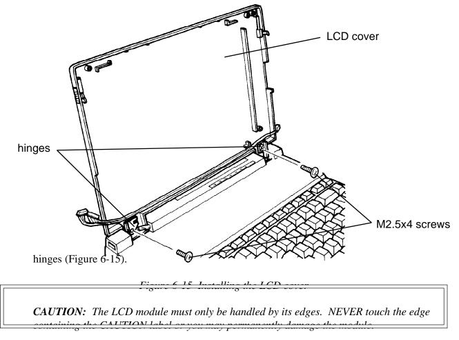
5. Place the LCD module in the LCD cover. Align the lower left corner of the LCD module
