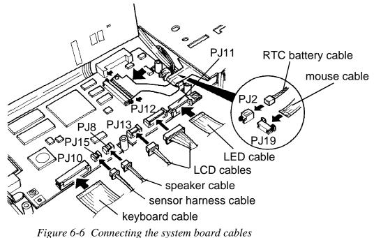
**CAUTION:** Route all cables so they will not be damaged when the middle base assembly is installed.
