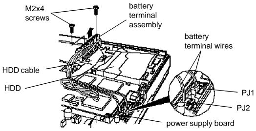
Figure 5-15 Removing the battery terminal assembly
