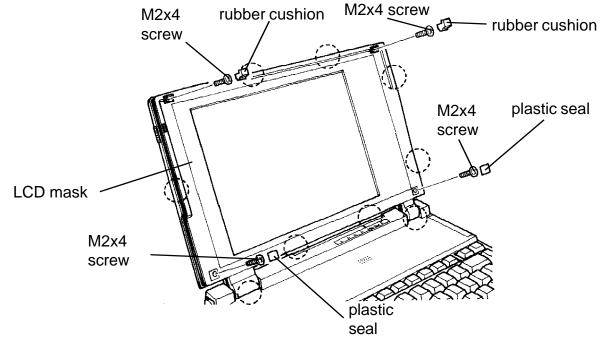
Figure 5-5 Removing the LCD rubber cushions, plastic seals, and screws
