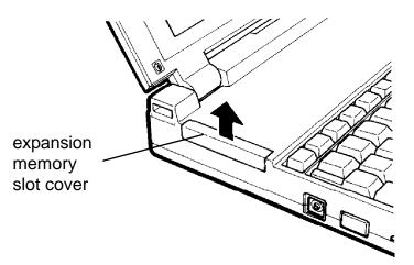
Figure 5-3 Removing the memory card slot cover
