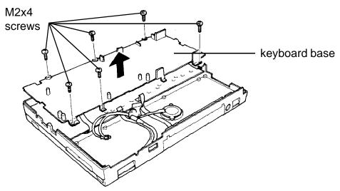
Figure 5-26 Removing the keyboard base
