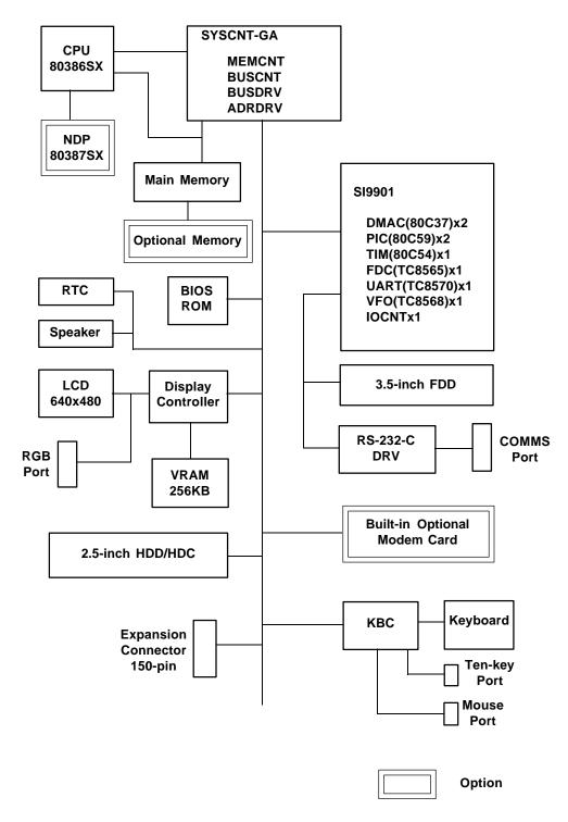
Figure 2-1 System unit block diagram
