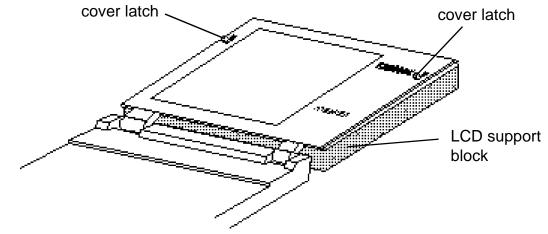
mask. If necessary, move the cover latches to position the LCD mask (Figure 6-19). Figure 6-19 Securing the latches on the LCD mask
