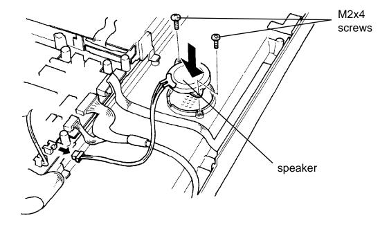
Figure 6-3 Securing the speaker
