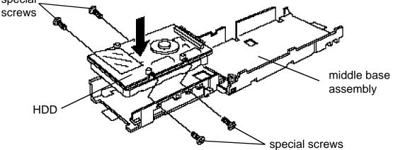
Figure 6-8 Securing the HDD to the middle base assembly
