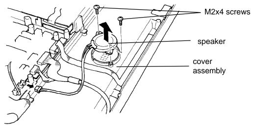
Figure 5-25 Removing the speaker
