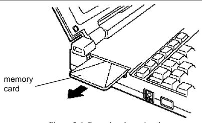
Figure 5-4 Removing the optional memory card
