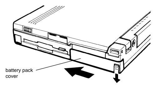
Figure 6-24 Installing the battery pack cover
