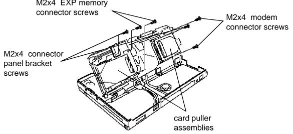
Figure 5-17 Removing the card modem and memory card connector screws
