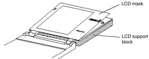
sure that the catch hook on the mask is secured with the tab (Figure 6-18).
