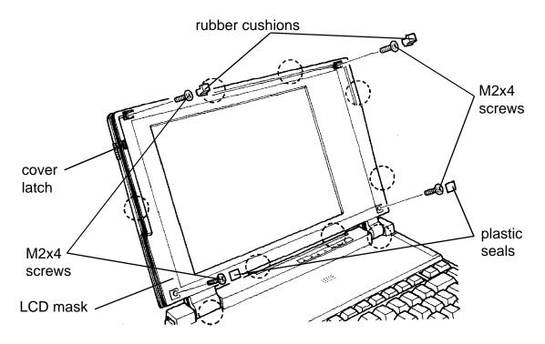
21. Insert the two rubber cushions and the two plastic seals on the LCD mask (Figure 6-21).
