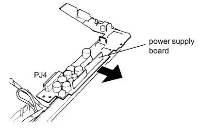
Figure 5-24 Removing the power supply board
