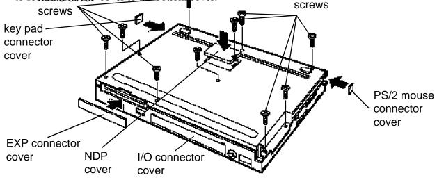
Figure 6-14 Installing the bottom cover screws
