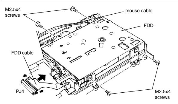
keyboard base as you remove the FDD. Figure 5-21 Removing the floppy disk drive
