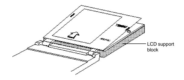
Figure 5-7 Releasing the bottom LCD mask latches
