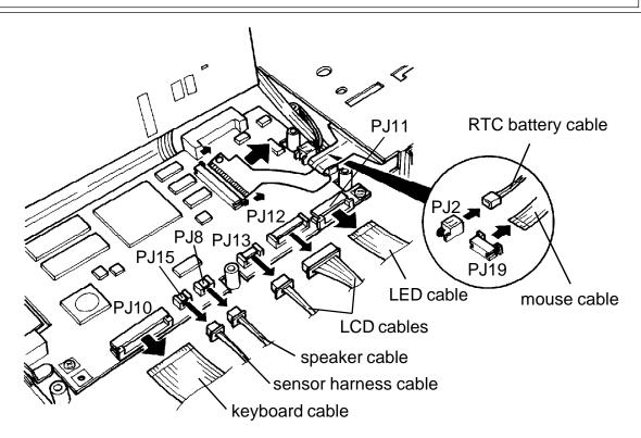
Figure 5-22 Disconnecting the cables from the system board
