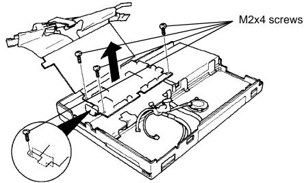
Figure 5-23 Removing the four system board screws
