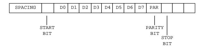
Figure 2-5 Start, parity, and stop bits
