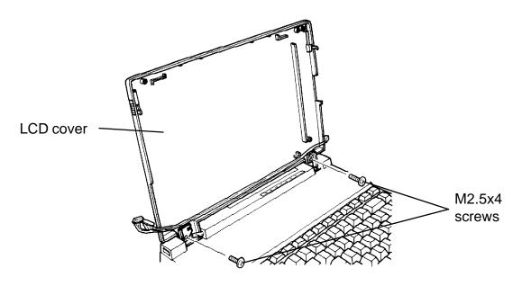
Figure 5-12 Removing the LCD cover
