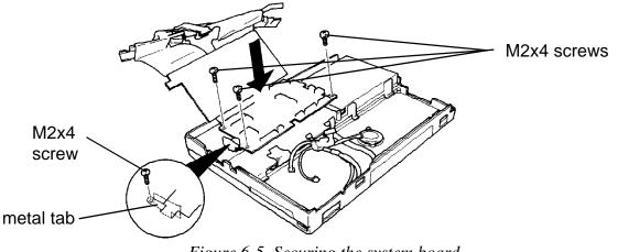
Figure 6-5 Securing the system board
