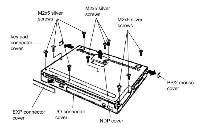
Figure 5-13 Removing the bottom cover screws
