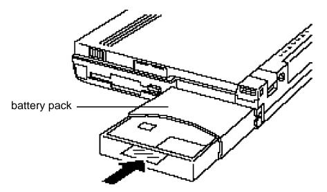
Figure 6-23 Inserting the battery pack
