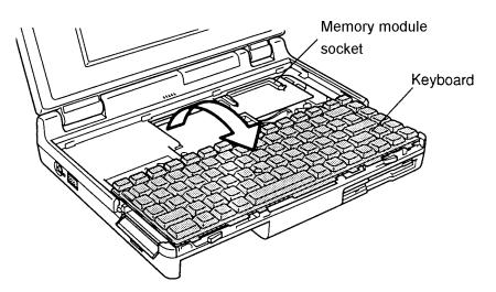
Figure 4-7 Exposing the Memory Module socket
