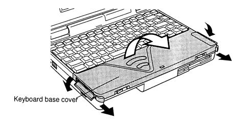
Figure 4-5 Removing the keyboard base cover
