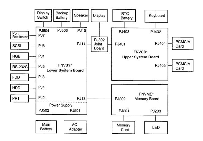
Figure 1-2 T2400CS/T2400CT system unit configuration
