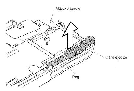
Figure 4-12 Removing the right side PCMCIA card ejector
