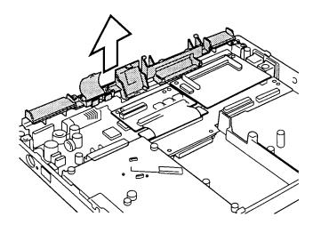
Figure 4-25 Removing the speaker/LED board/backup battery table frame
