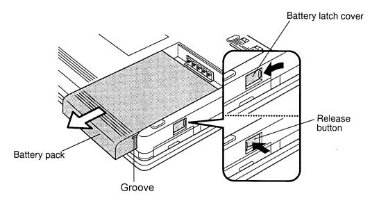
Figure 4-1 Removing the battery pack
