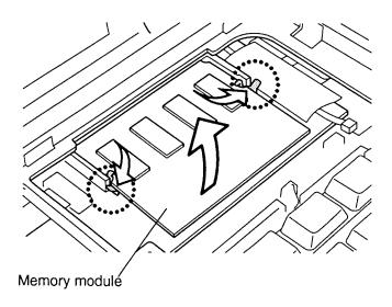
Figure 4-8 Removing the memory module
