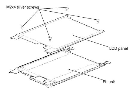
Figure 4-32 Removing the FL screws
