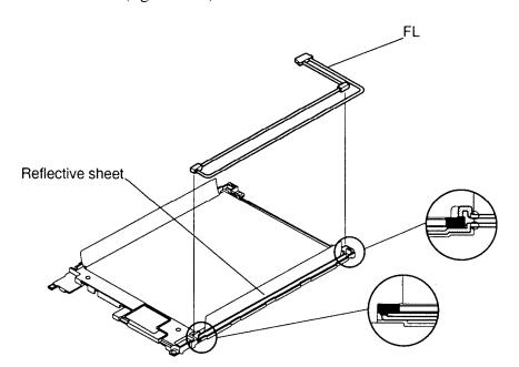
Figure 4-33 Removing the FL
