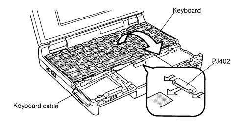
Figure 4-6 Removing the keyboard
