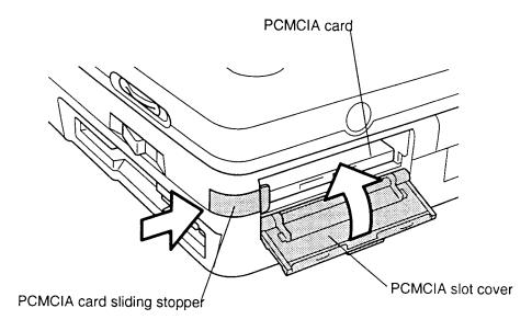
Figure 4-3 Installing the optional PCMCIA card
