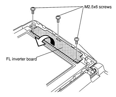
Figure 4-28 Removing the FL inverter board
