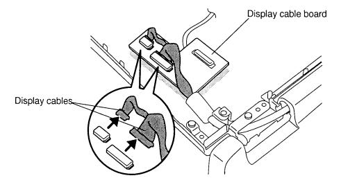
Figure 4-38 Removing the display cable board
