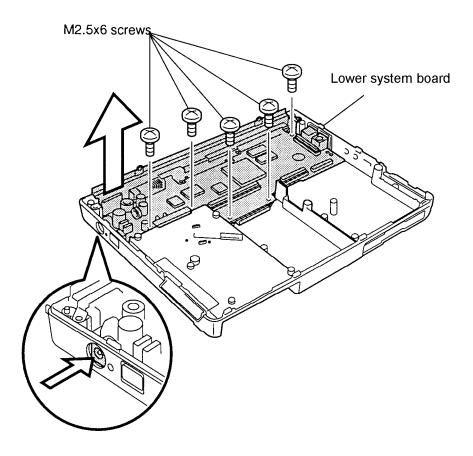
Figure 4-27 Removing the lower system board
