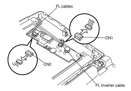
Figure 4-29 Disconnecting the FL inverter board
