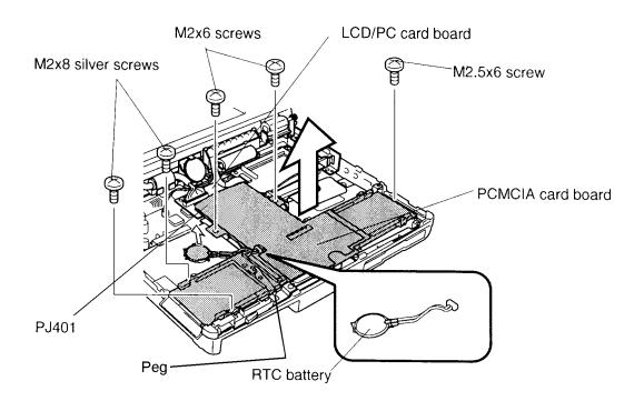
Figure 4-13 Removing the RTC battery and upper system board
