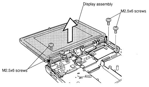
Figure 4-23 Removing the display assembly
