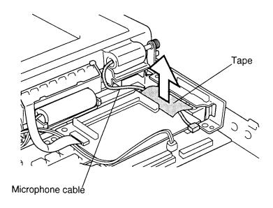
Figure 4-18 Peeling off the tape
