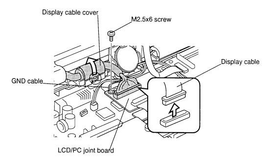
Figure 4-22 Disconnecting the display cable
