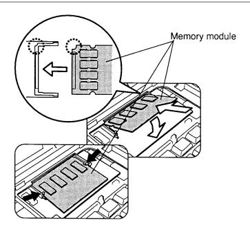
Figure 4-9 Inserting the memory module
