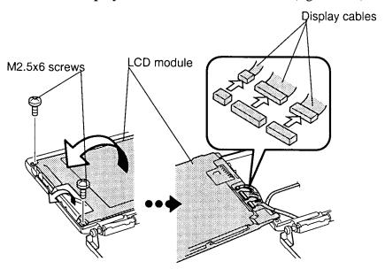
Figure 4-30 Removing the LCD module
