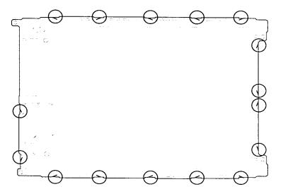
Figure 4-31 Unbending the color LCD module latches
