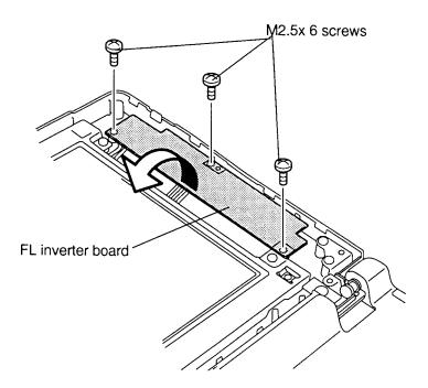
Figure 4-34 Removing the FL inverter board
