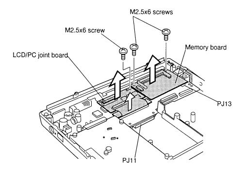
Figure 4-26 Removing the memory board and LCD/PC card joint board
