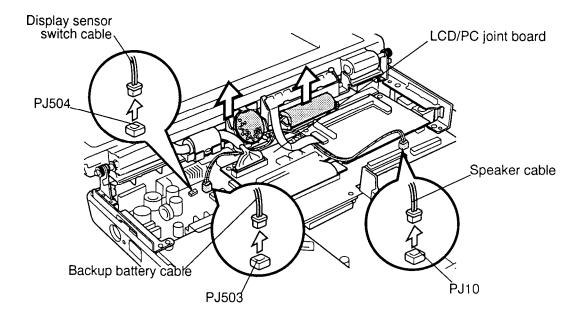
Figure 4-21 Removing the cable
