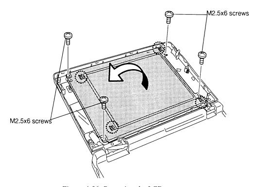
Figure 4-36 Removing the LCD screws
