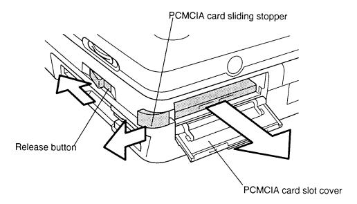
Figure 4-2 Removing the PCMCIA card
