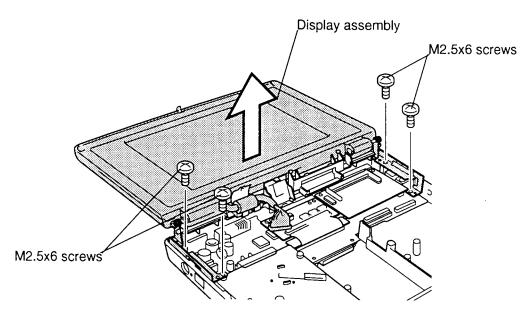
Figure 4-23 Removing the display assembly
