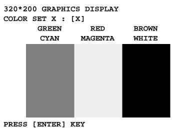
Pressing **Enter** toggles between tests. To exit this subtest and return to the DISPLAY TEST menu, press **Ctrl + Break**.
