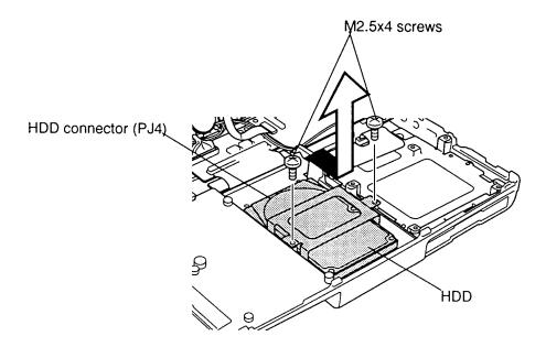
Figure 4-14 Removing the HDD with bracket
