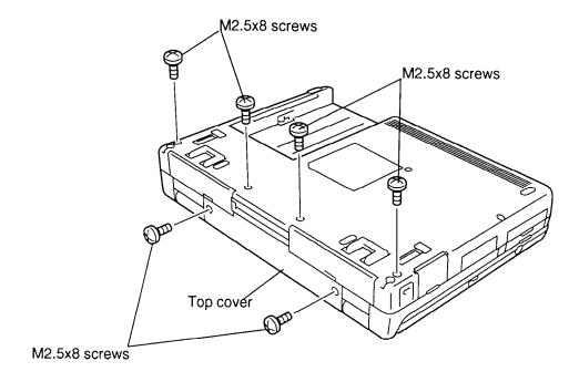
Figure 4-10 Removing top cover screws
