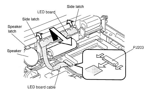
Figure 4-24 Removing the LED board
