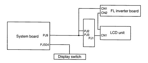
Figure 2-4 T2400CT display connection
