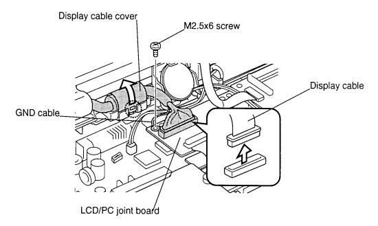
Figure 4-22 Disconnecting the display cable
