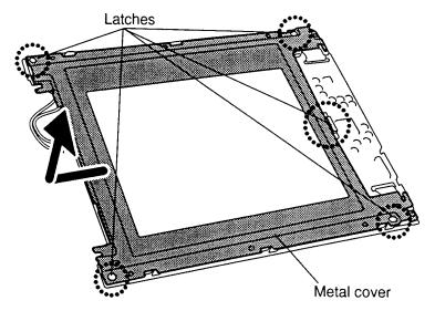
Figure 4-40 Removing the metal cover.
