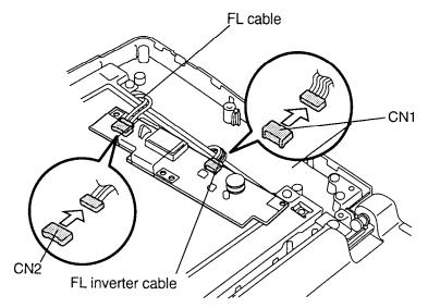
Figure 4-35 Disconnecting the FL inverter board
