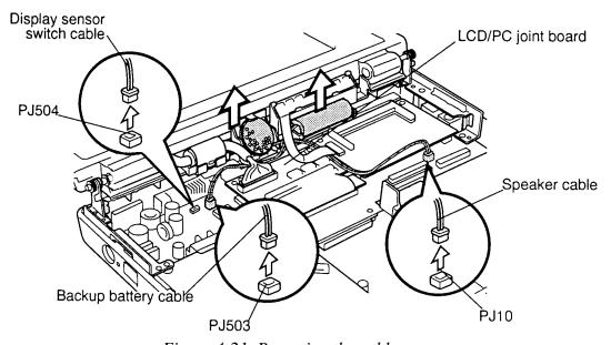
Figure 4-21 Removing the cable
