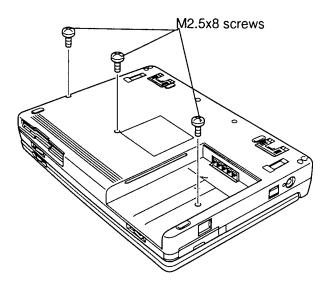
Figure 4-4 Removing three screws
