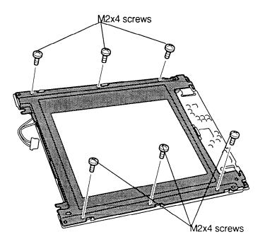
Figure 4-39 Removing the FL screws
