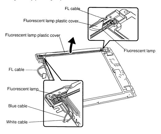
Figure 4-41 Removing the fluorescent lamp
