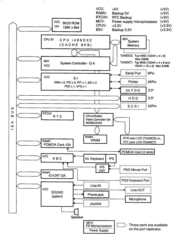
Figure 1-3 T2400CS/T2400CT system board block diagram
