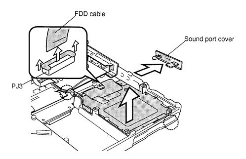
Figure 4-16 Removing the FDD with bracket
