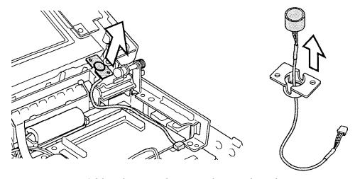
Figure 4-20 Lifting out the internal microphone base
