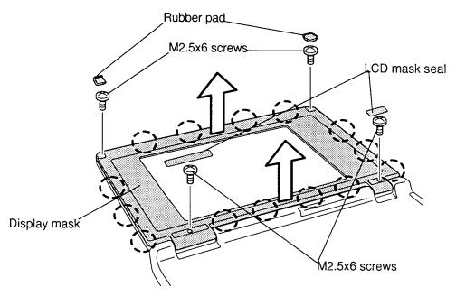
Figure 4-19 Removing the display mask
