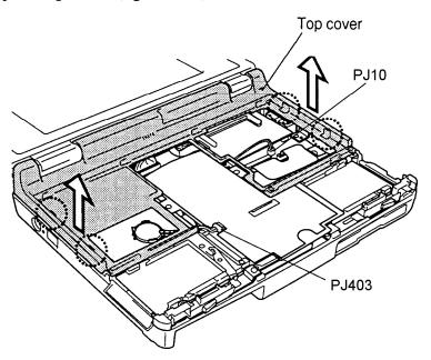
Figure 4-11 Unlatching the top cover
