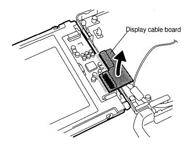
Figure 4-37 Removing the LCD module
