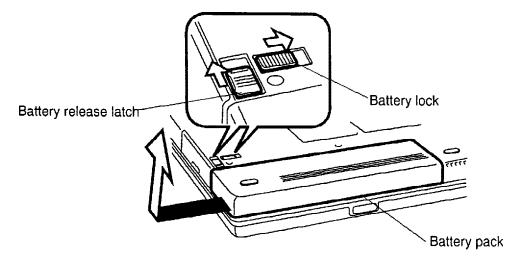
Figure 4-1 Unlocking the battery pack
