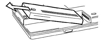
Figure 4-2 Lifting out the battery pack
