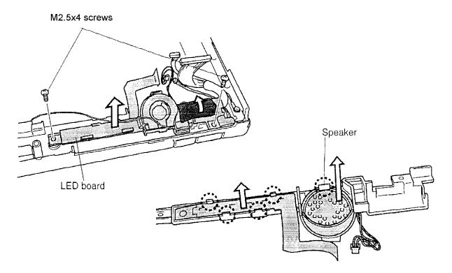
Figure 4-24 Removing the LED board
