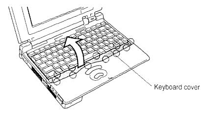
Figure 4-9 Unlatching the keyboard cover
