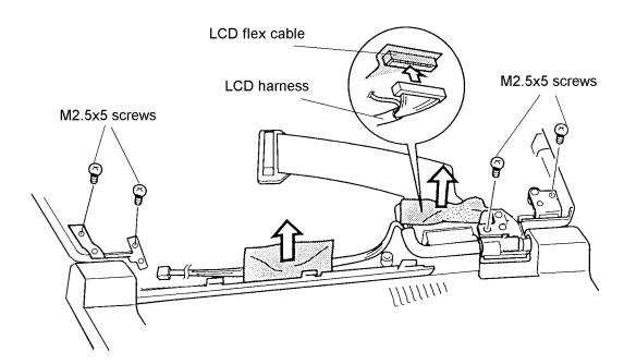
Figure 4-31 Removing the display cable
