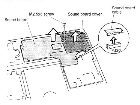
Figure 4-20 Removing the sound board
