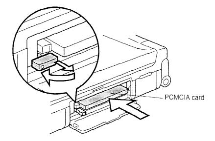
Figure 4-8 Installing the PCMCIA card
