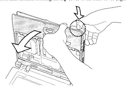
Figure 4-17 Separating the top cover
