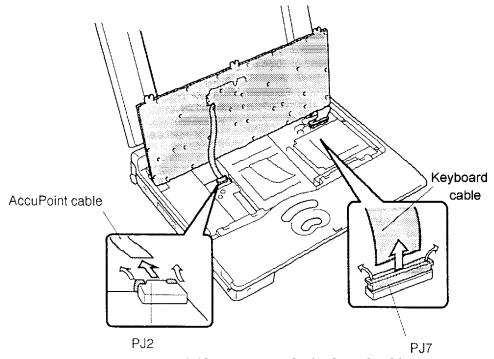
Figure 4-12 Removing the keyboard cable
