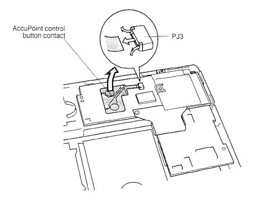
Figure 4-19 Removing the AccuPoint control button contact
