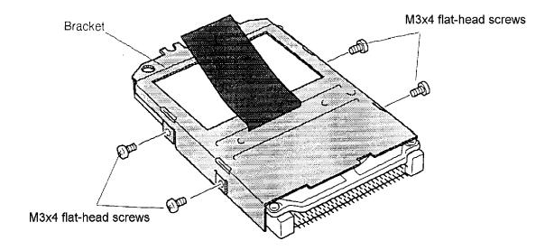
Figure 4-14 Removing the HDD bracket
