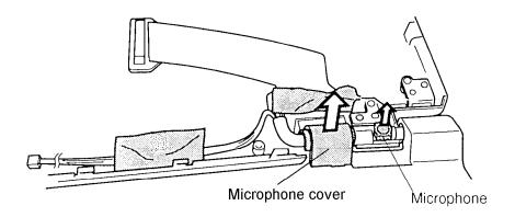
Figure 4-30 Removing the microphone
