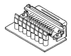
Figure 2-2 Printer port LED
