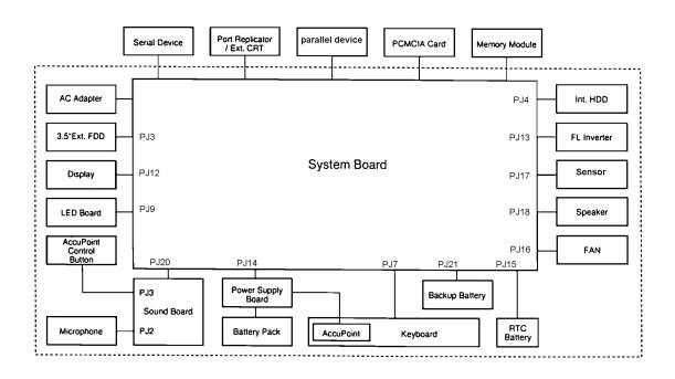
Figure 1-2 610CT system unit configuration
