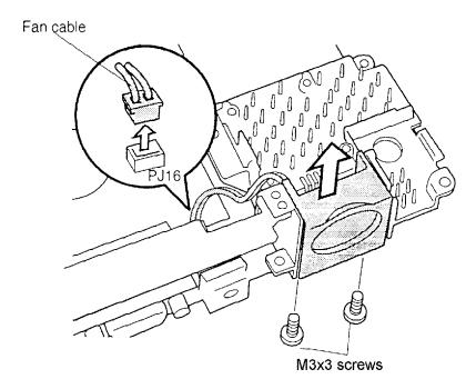
Figure 4-23 Removing the fan
