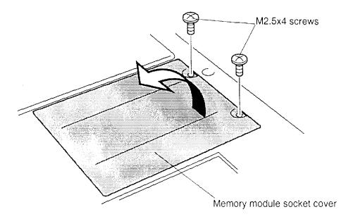
Figure 4-4 Removing the memory module socket cover
