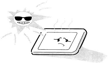
8. Do not store the module at temperatures below specifications. Cold can cause the liquid crystals to freeze, lose their elasticity or otherwise suffer damage.
