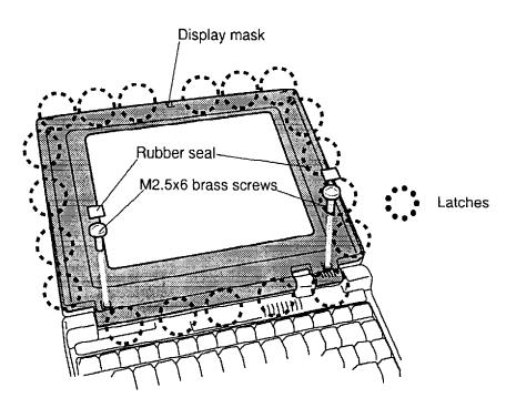
Figure 4-25 Removing the display mask
