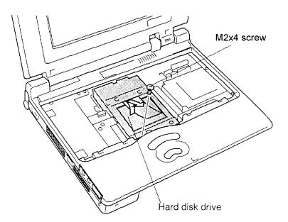
Figure 4-13 Removing the HDD with bracket
