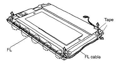
Figure 4-29 Removing the FL
