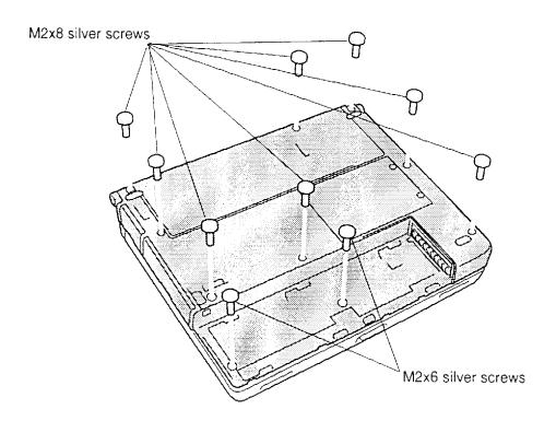
Figure 4-15 Removing the bottom cover screws
