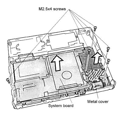
Figure 4-22 Removing the system board
