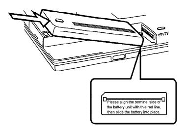
Figure 4-3 Installing the battery pack
