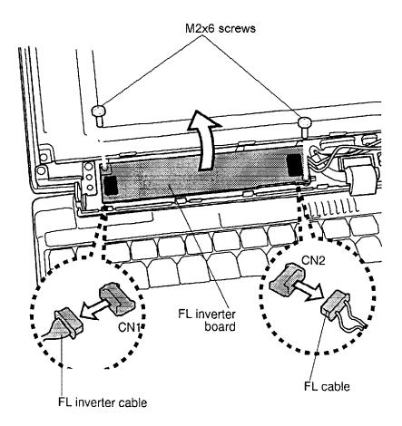
Figure 4-26 Removing the FL inverter board
