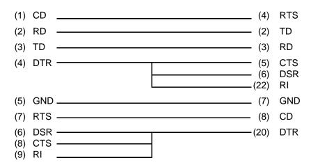
Figure F-4 RS-232-C direct cable (9-pin to 25-pin)
