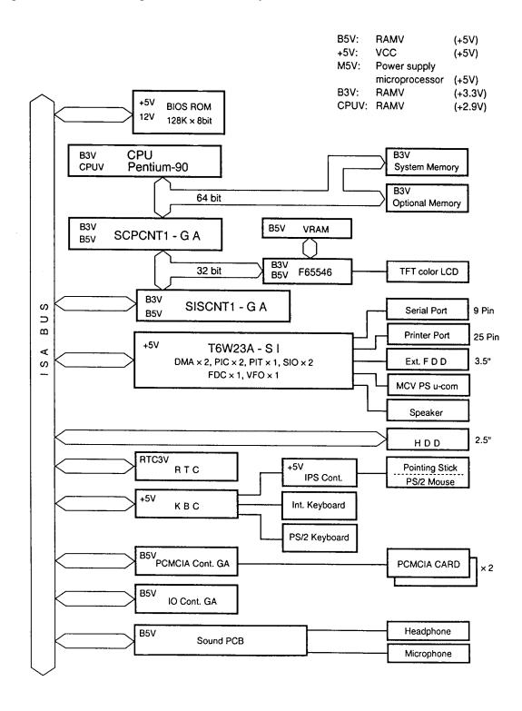
Figure 1-3 610CT system board block diagram
