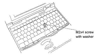
Figure 4-10 Removing one keyboard screw
