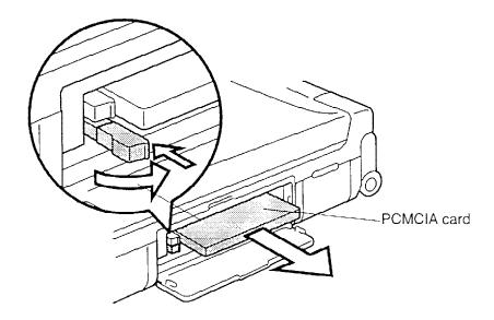
Figure 4-7 Removing the PCMCIA card
