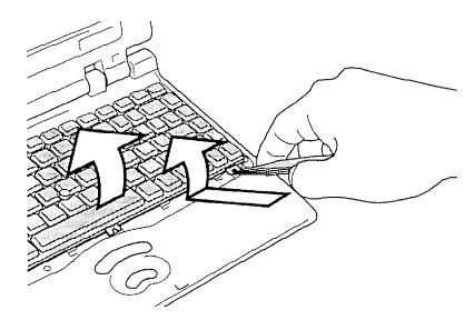
Figure 4-11 Lifting the keyboard
