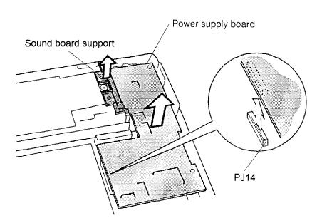
Figure 4-21 Removing the power supply board
