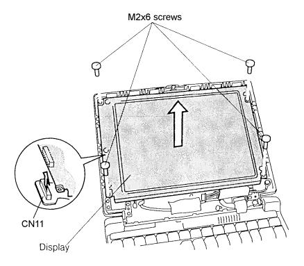
Figure 4-27 Removing the display module screws
