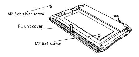
Figure 4-28 Removing the FL unit screws
