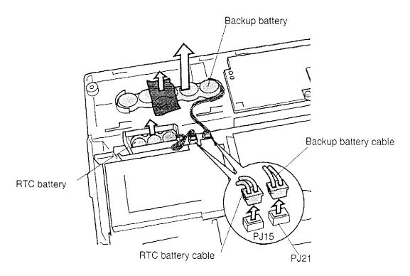
Figure 4-18 Removing the RTC and backup batteries
