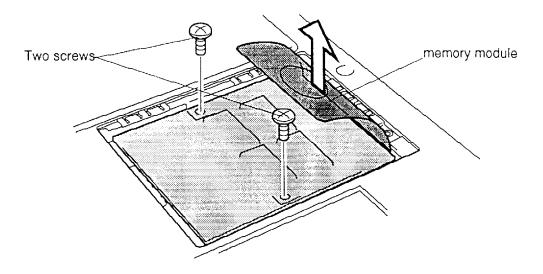
Figure 4-5 Removing the memory module
