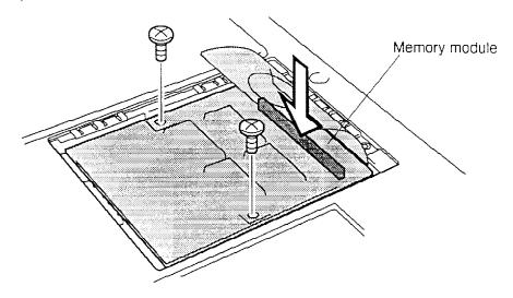
Figure 4-6 Inserting the memory module
