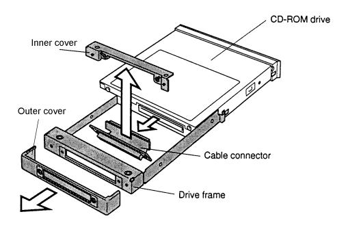
Figure 4-15 Removing the CD-ROM drive
