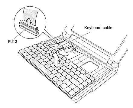
Figure 4-20 Removing the keyboard
