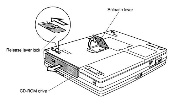
Figure 4-13 Removing the CD-ROM drive module
