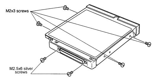
Figure 4-14 Removing the screws
