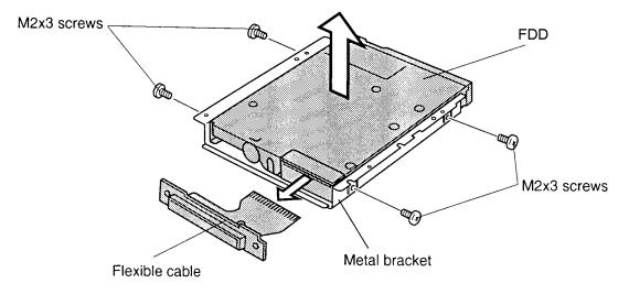
Figure 4-12 Removing the FDD
