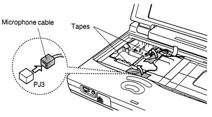
Figure 4-23 Disconnecting the microphone cable
