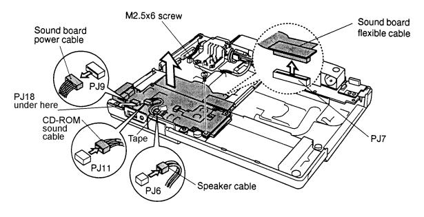
Figure 4-32 Removing the sound board
