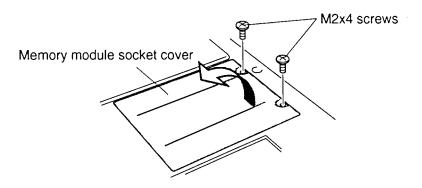
Figure 4-6 Removing the memory module socket cover
