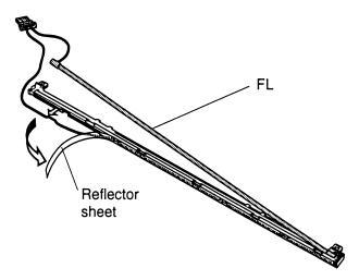
Figure 4-52 Removing the FL (DSTN)
