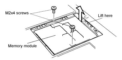
Figure 4-7 Removing the memory module
