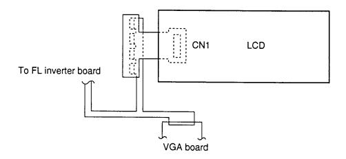
Figure 2-4 200CDT display connection
