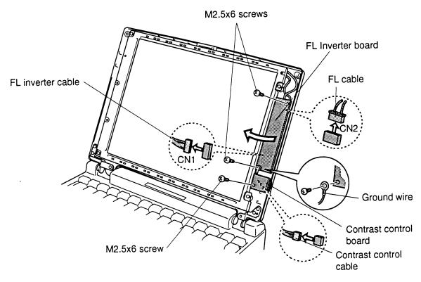
Figure 4-44 Removing the FL inverter board (DSTN)
