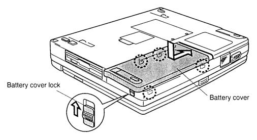
Figure 4-3 Installing the battery pack cover
