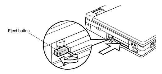
Figure 4-5 Installing the PC card
