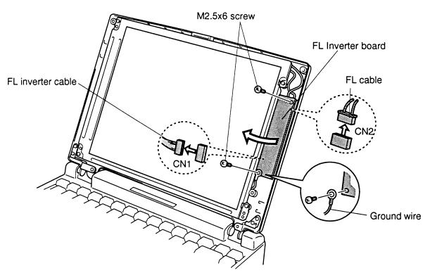
Figure 4-43 Removing the FL inverter board (TFT)
