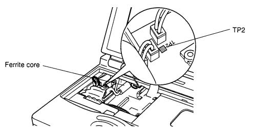
Figure 4-26 Measuring the voltage at TP2
