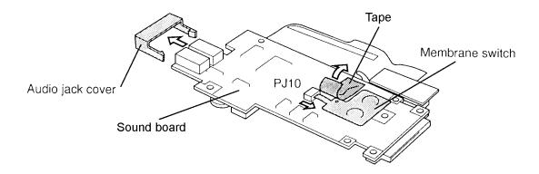
Figure 4-33 Removing the membrane switch
