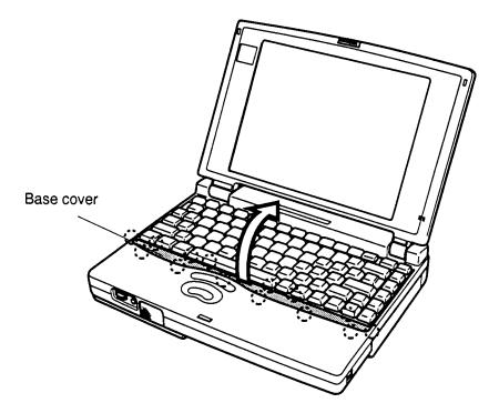
Figure 4-18 Removing the keyboard base
