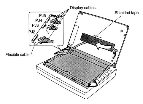
Figure 4-46 Removing the LCD module (TFT)
