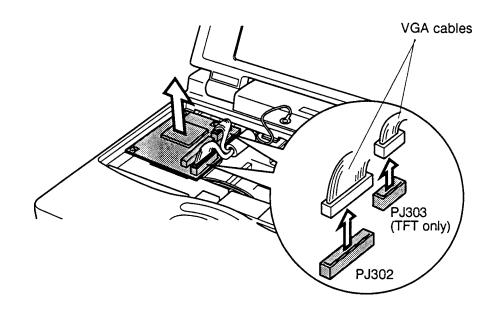
Figure 4-25 Disconnecting the cables from the VGA board
