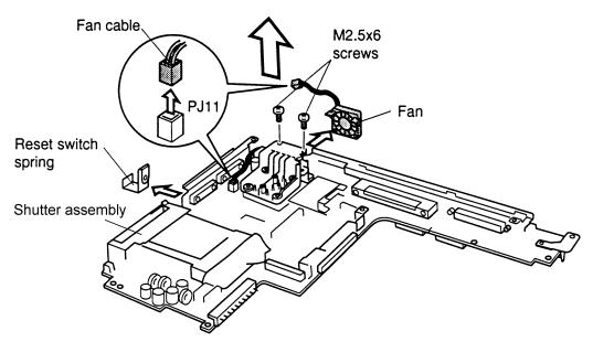
Figure 4-40 Removing the fan
