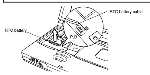
Figure 4-28 Removing the RTC battery
