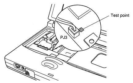
Figure 4-30 Measuring the voltage at PJ3
