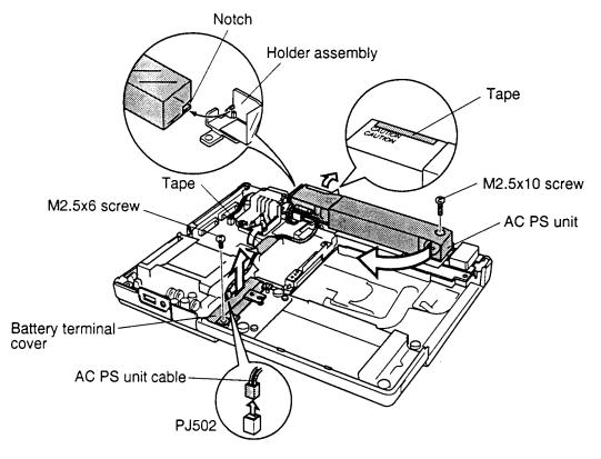
6. Turn the **AC PS unit** out of its seating and lay it on its side.
