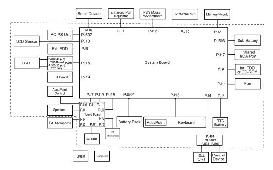
Figure 1-2 200 series system unit configuration
