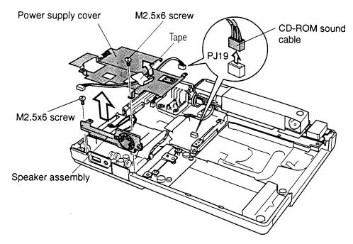
Figure 4-34 Removing the speaker assembly
