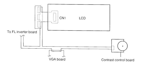
Figure 2-3 200CDS display connection
