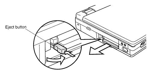
Figure 4-4 Removing the PC card
