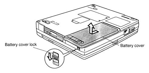
Figure 4-1 Removing the battery pack cover
