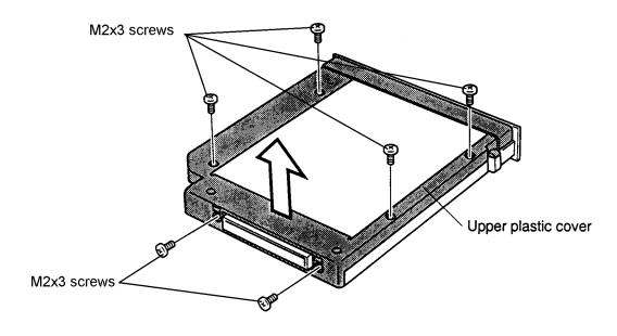
Figure 4-10 Removing the screws
