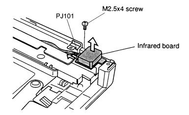
Figure 4-38 Removing the infrared board
