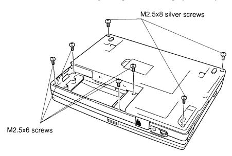
Figure 4-27 Removing the top cover screws
