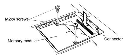
Figure 4-8 Installing the memory module
