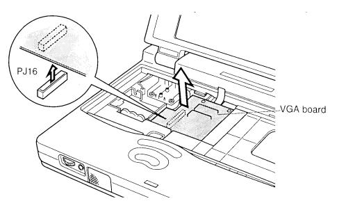
Figure 4-24 Disconnecting the VGA board
