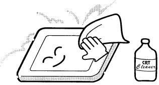
4. If water or other liquid is left on the panel's surface for a long period, it can change the screen's tint or stain it. Be sure to quickly wipe off any liquid.
