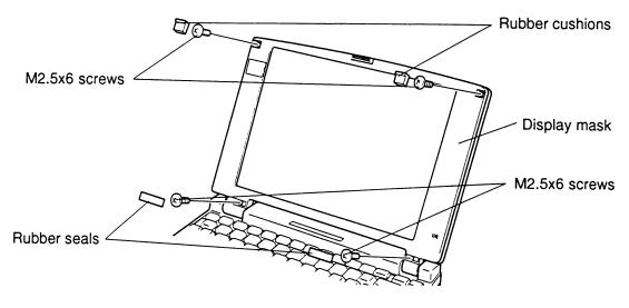
Figure 4-41 Removing the rubber seals, cushions, and screws
