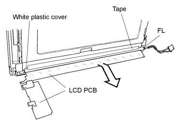
Figure 4-50 Removing the FL (TFT)
