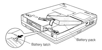
*Figure 4-2 Removing the battery pack*
