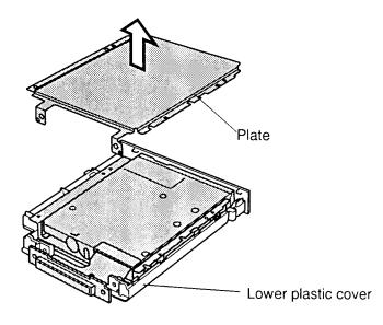
Figure 4-11 Removing the plate
