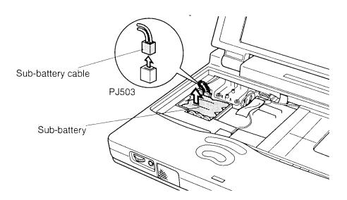
Figure 4-22 Removing the sub-battery
