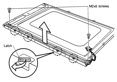
Figure 4-51 Removing the FL assembly (DSTN)
