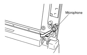
Figure 4-53 Removing the microphone
