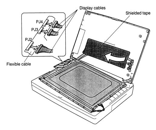
7. Remove the **shielded tape** securing the display cables to the LCD cover.
