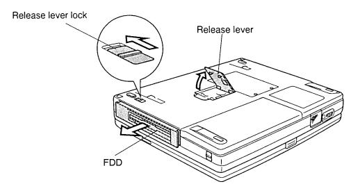
Figure 4-9 Removing the FDD module
