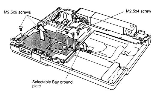
4. Remove the **sound board cover** with **Selectable Bay ground plate**.
