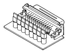
Figure 2-2 Printer port LED
