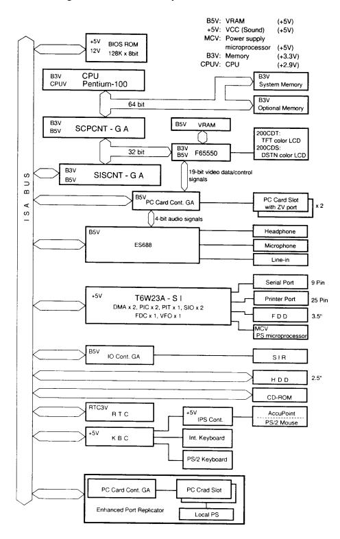
Figure 1-3 200 series system board block diagram
