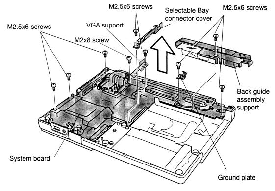
Figure 4-39 Removing the system board
