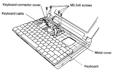
Figure 4-19 Removing the metal cover
