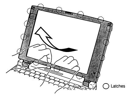
Figure 4-42 Removing the display mask
