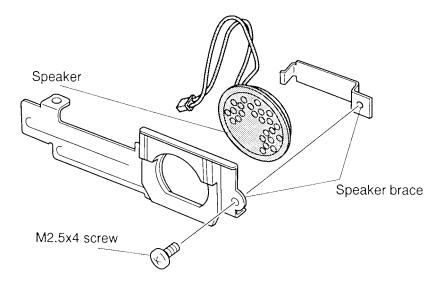
Figure 4-35 Removing the speaker
