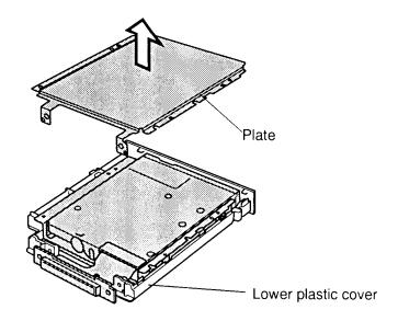
Figure 4-11 Removing the plate and lower plastic cover
