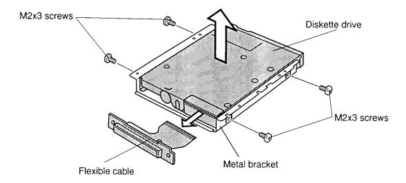
Figure 4-12 Removing the diskette drive
