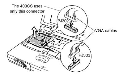
Figure 4-23 Disconnecting the cables from the VGA board
