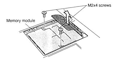
*Figure 4-7 Removing the memory module*
