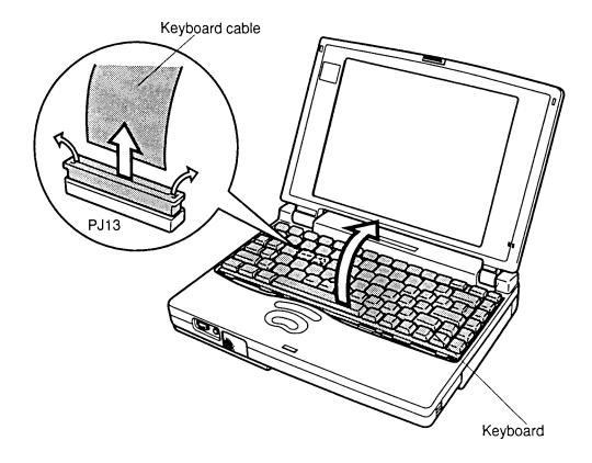
Figure 4-19 Removing the keyboard
