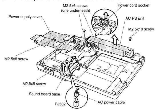
Figure 4-29 Removing the AC PS unit
