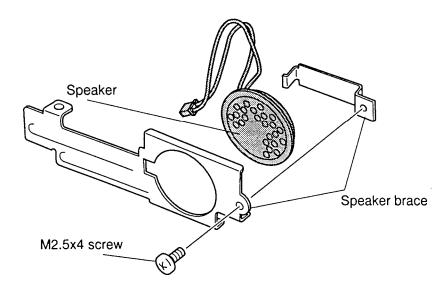
Figure 4-32 Removing the speaker
