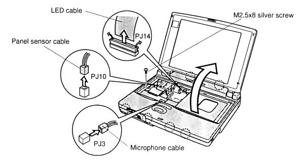
Figure 4-26 Removing the top cover and display assembly
