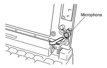
Figure 4-45 Removing the microphone
