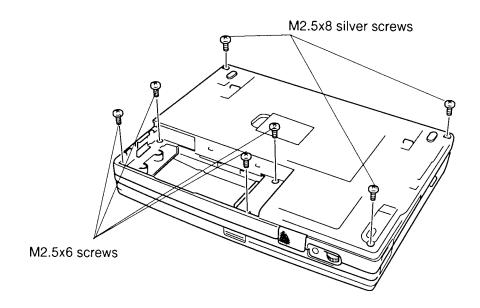
Figure 4-24 Removing the top cover screws
