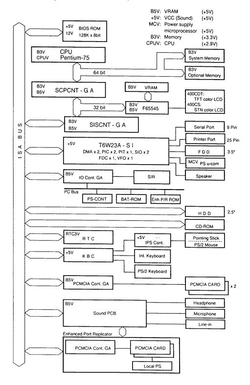
Figure 1-3 400 series system board block diagram
