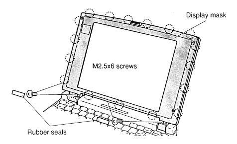
Figure 4-35 Removing the display mask
