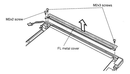
Figure 4-43 Removing the 400CDT FL cover
