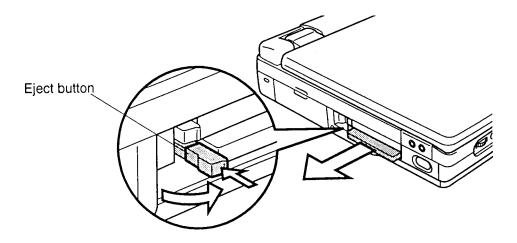
Figure 4-4 Removing the PCMCIA card
