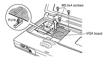
Figure 4-22 Removing the VGA board
