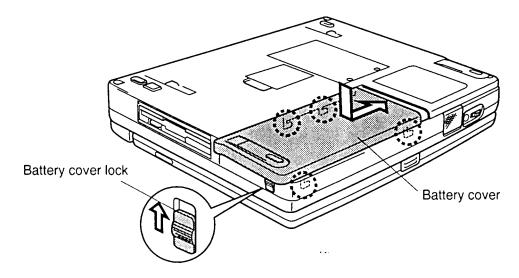
Figure 4-3 Installing the battery pack
