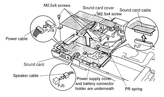
Figure 4-27 Removing the sound card
