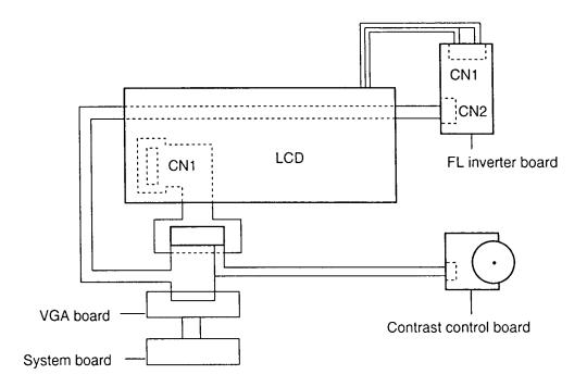
Figure 2-3 400CS display connection
