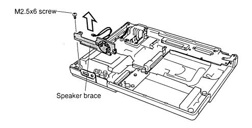
Figure 4-31 Removing the speaker brace
