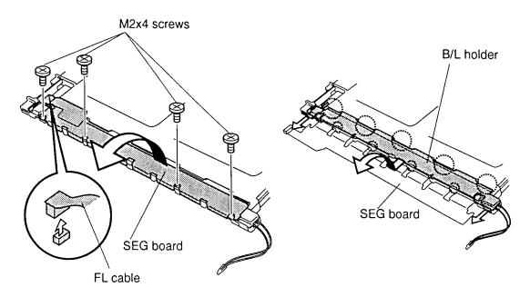
Figure 4-40 Removing SEG board screws
