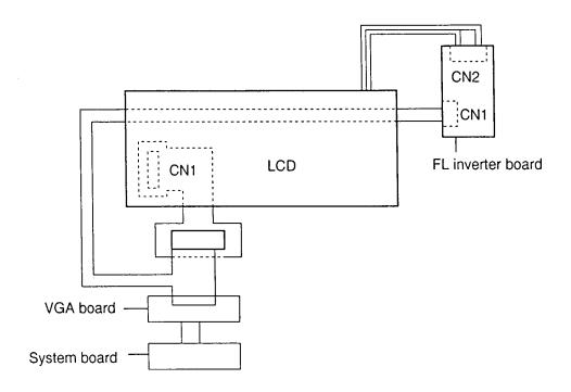
Figure 2-4 400CDT display connection
