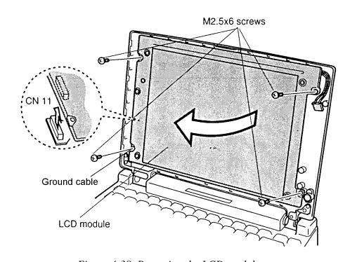
Figure 4-38 Removing the LCD module
