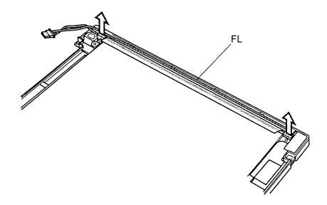
Figure 4-44 Removing the 400CDT FL
