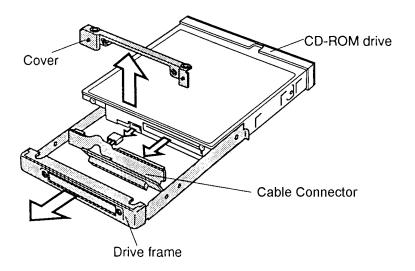
Figure 4-15 Removing the CD-ROM
