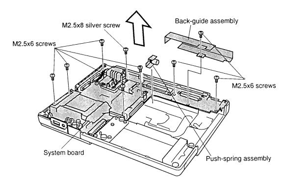
Figure 4-33 Removing the system board
