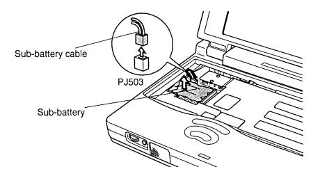
*Figure 4-20 Removing the sub-battery*
