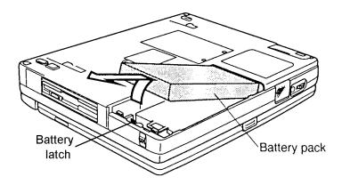
Figure 4-2 Removing the battery pack
