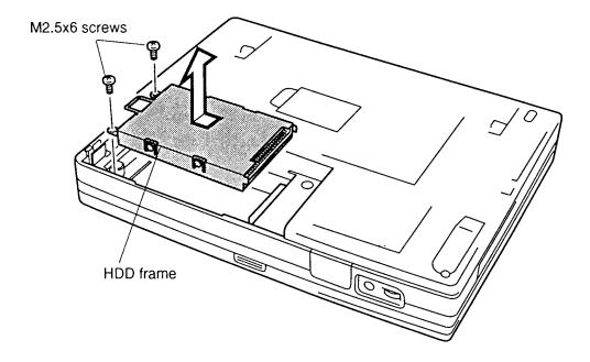
Figure 4-16 Removing the frame with the HDD
