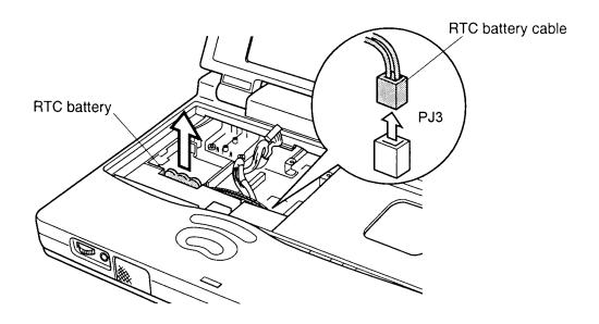
Figure 4-25 Removing the RTC battery
