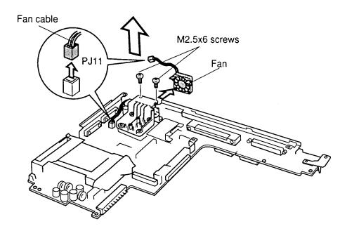
Figure 4-34 Removing the fan
