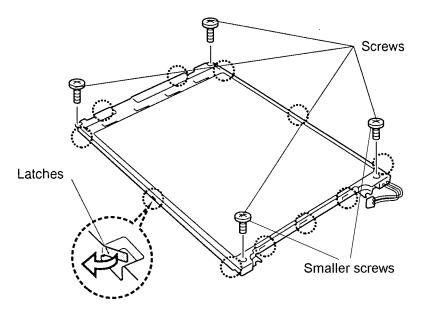
Figure 4-39 Unbending the color LCD module latches and removing screws
