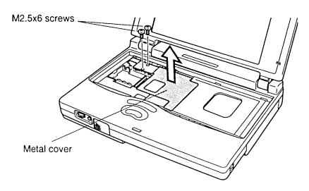
Figure 4-21 Removing the metal cover
