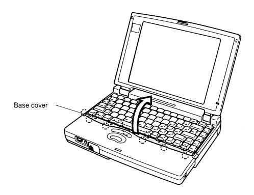
Figure 4-18 Removing the keyboard base
