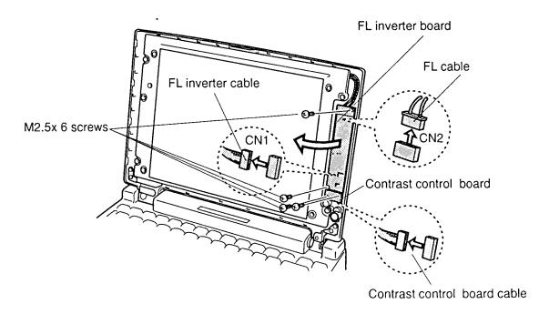
Figure 4-36 Removing the 400CS FL inverter board
