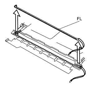
Figure 4-42 Lifting the end of the reflector sheet
