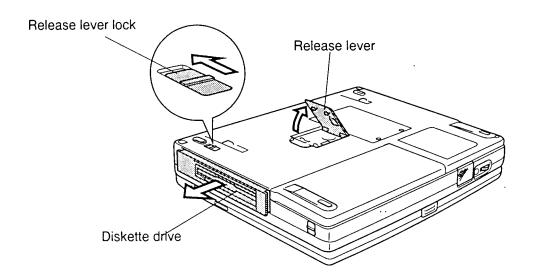
Figure 4-9 Removing the diskette drive
