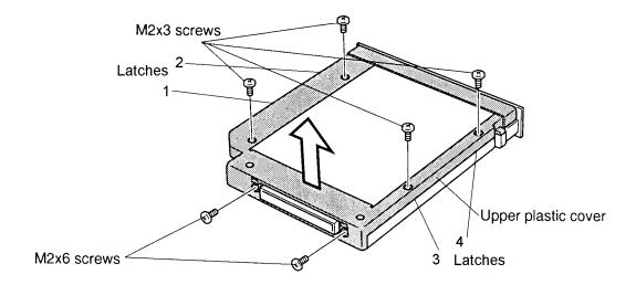
Figure 4-10 Removing the upper plastic cover
