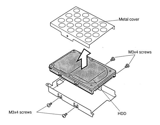
Figure 4-17 Removing the HDD from the frame
