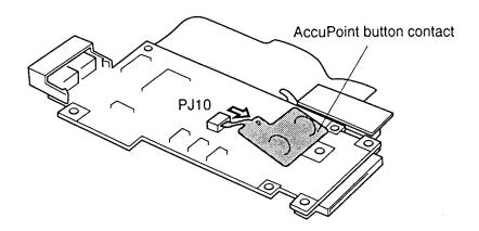
Figure 4-28 Removing the AccuPoint button contact
