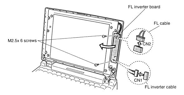
Figure 4-37 Removing the 400CDT FL inverter board
