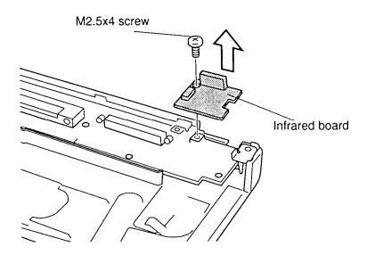
Figure 4-30 Removing the infrared board
