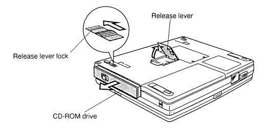
Figure 4-13 Removing the CD-ROM drive
