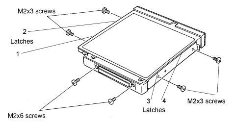
Figure 4-14 Removing the frame
