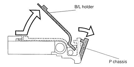
Figure 4-41 Disconnecting the B/L holder
