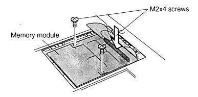
Figure 4-8 Inserting the memory module
