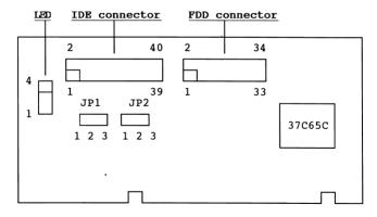
JP1: IOCS16 line with or without buffer output. . Set 1-2 with buffer output.
